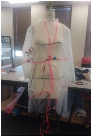
I planned the layout of the wire ahead of time by draping the wire around the jacket. The five separate pieces all connect to two battery packs concealed within the pocket. One battery pack is capable of powering the entire jacket, but I chose to divide it between two battery packs for display purposes. This way, each pack could run for a longer period of time without needing the batteries replaced.
