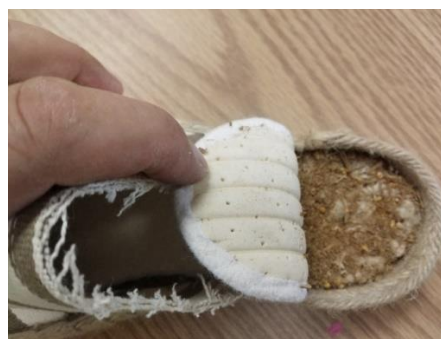
(b) The mycelium composite midsole
