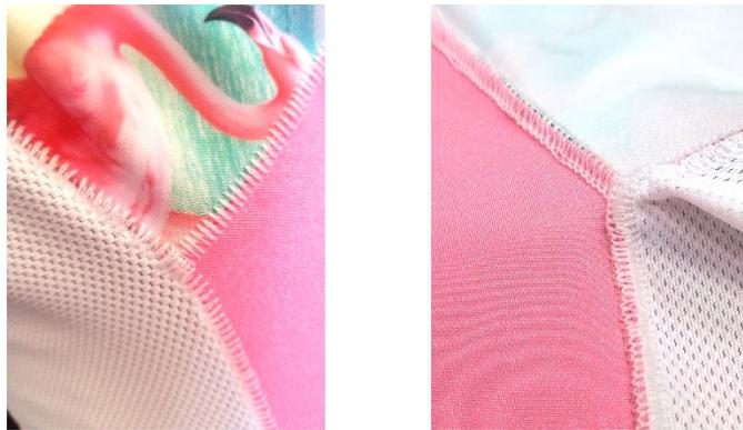
Figure 1. ActiveSeam™ seam joining areas (exterior and interior).
