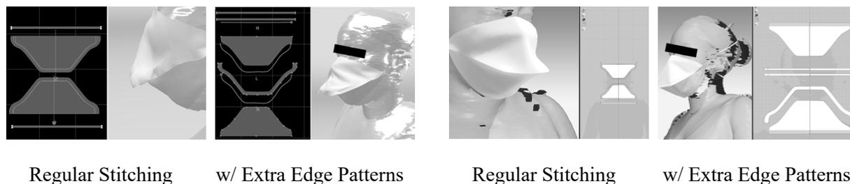
Fig. 4. Stitching results with Halyard mask (left, Browzwear & right, CLO).
