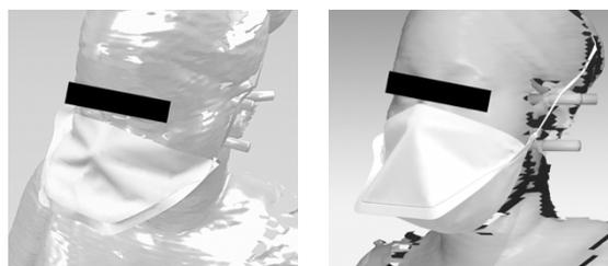
Fig. 3. Results of material physics with Halyard mask (left, Browzwear & right, CLO).
