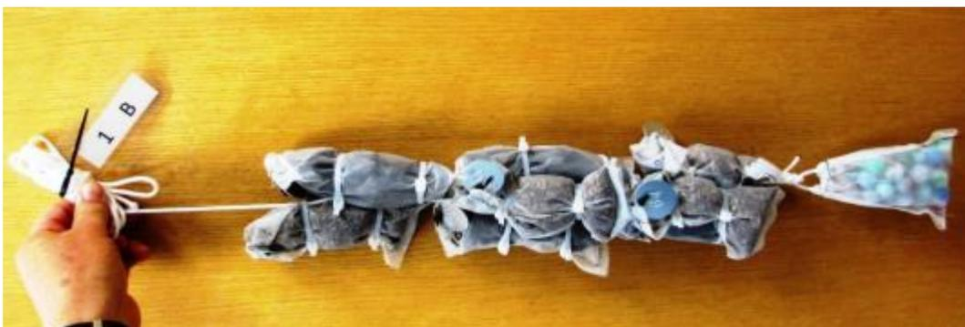
Figure 2. Wood chip sampling bag assembly image.
