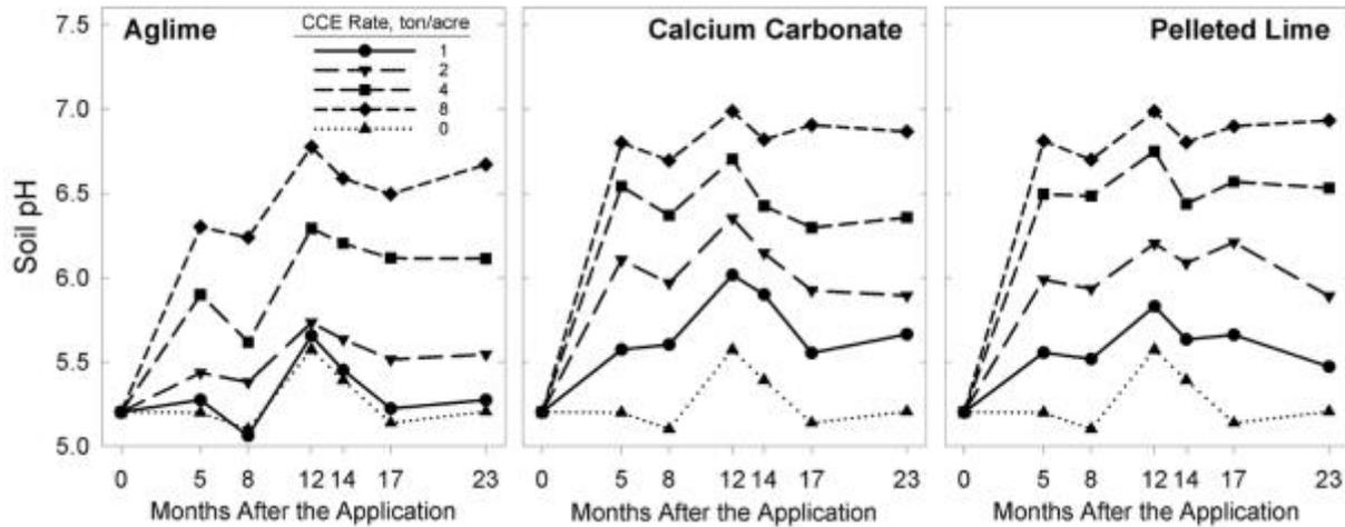
Figure 1. Effect of several calcium carbonate equivalent (CCE) application rates with three lime sources on soil pH over a 23-month period (averages across two sites).
