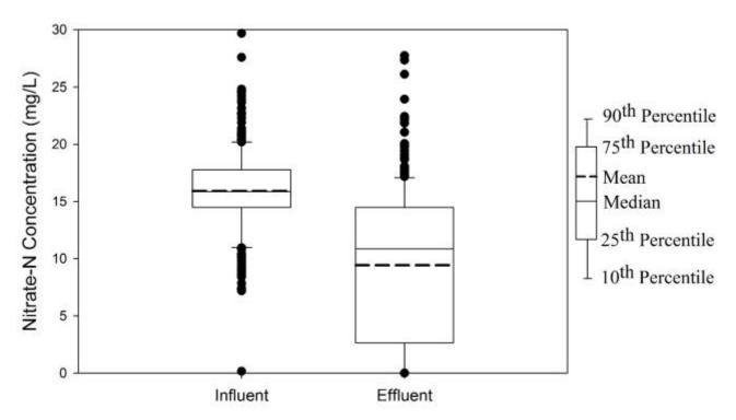
Figure 1. Box plot of nitrate-N concentrations in the influent and effluent from the bioreactor for 2012-2016.
