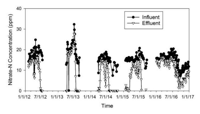
Figure 1. Nitrate-N concentrations in the bioreactor influent and effluent.
