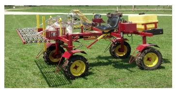
Figure 2. Self-propelled research sprayer built by Iowa State personnel.
