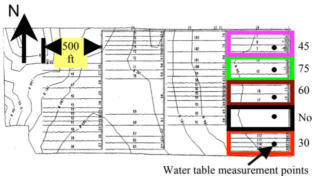
**Figure 1. Tile spacing study layout.**
