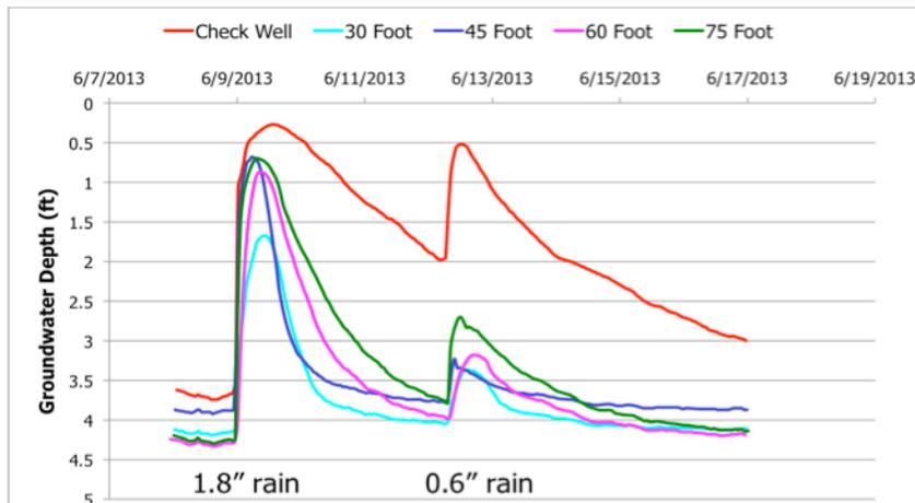
Figure 3. 2009 water table drawdown rates by tile spacing.
