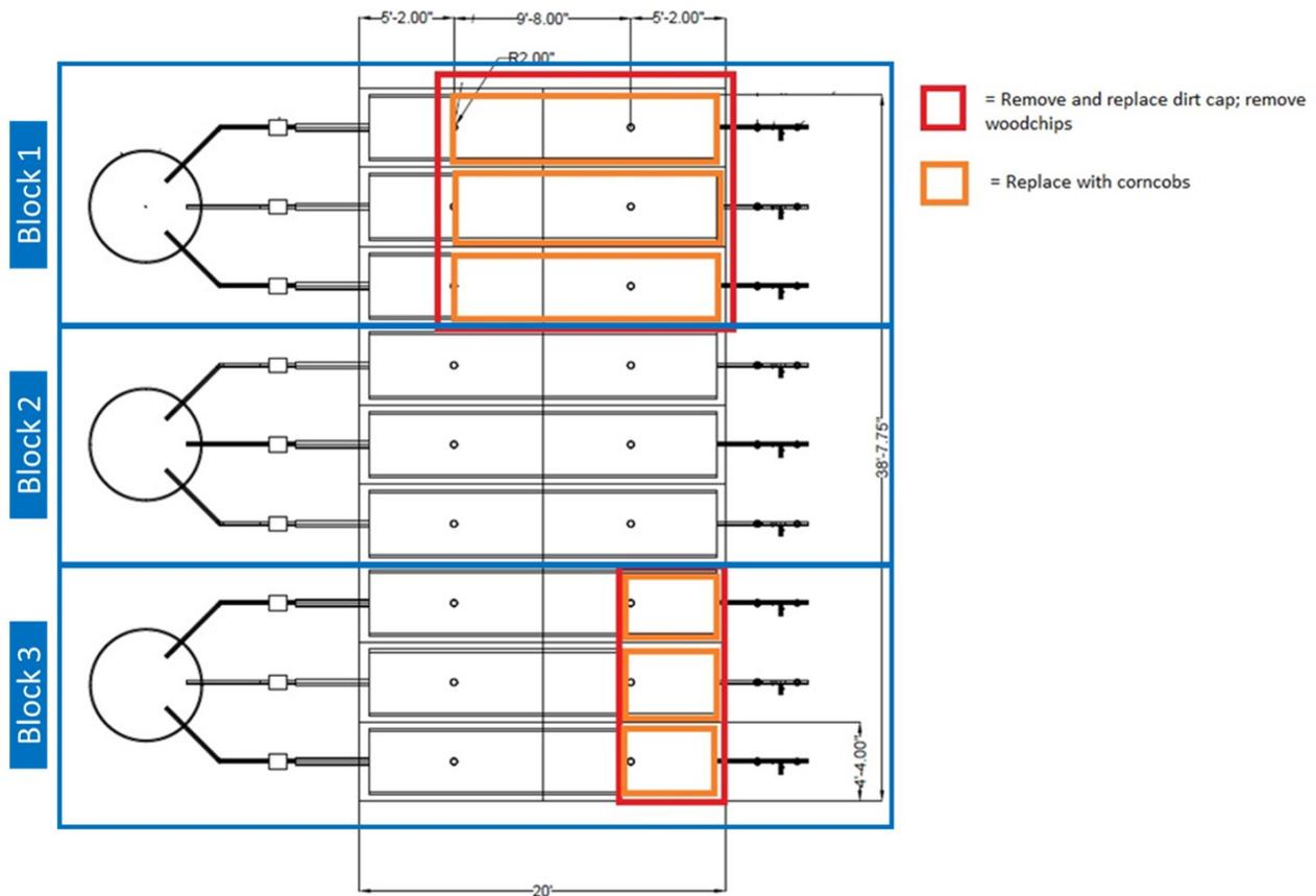
**Figure 1. Schematic of the excavation and corn cob refill plan for the pilot-scale bioreactors. Block 2 was maintained as the woodchip filled control; block 1 was excavated to 3/4 the bioreactor length and refilled with corn cobs; block 3 was excavated to 1/4 bioreactor length and refilled with corn cobs.**
