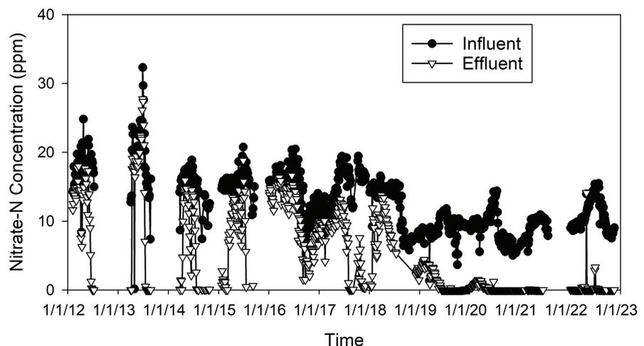
Figure 1. Nitrate-N concentrations in the bioreactor influent and effluent from 2012-2022
