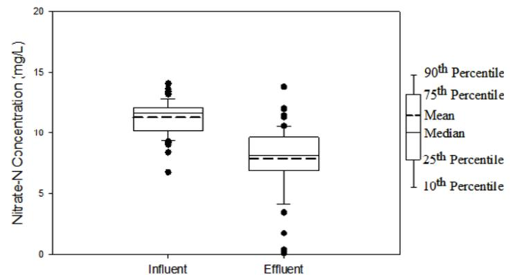
Figure 3. Box plot of nitrate-N concentrations in the influent and effluent from the bioreactor for 2019-2022.
