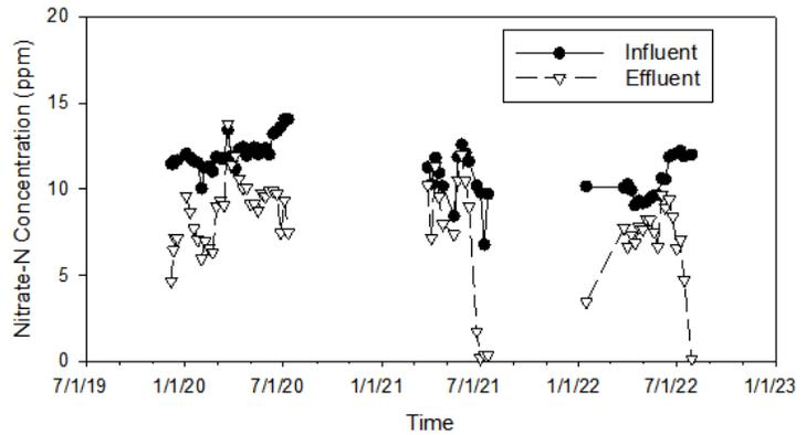
Figure 2. Time-series of nitrate-N concentrations in the influent and effluent from the bioreactor for 2019-2022.
