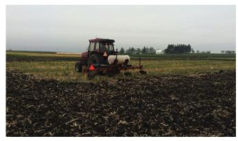
Figure 1. Side-dresser used for applying liquid UAN to Miscanthus plots prior to planting.
