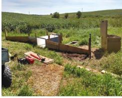
Figure 2. Flume structure for monitoring runoff.
