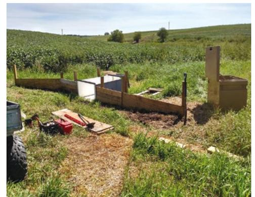
Figure 2. Flume structure for monitoring runoff.
