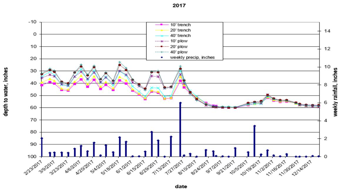
Figure 1. Water table and weekly precipitation in 2017 from two drainage installation methods at three distances.
