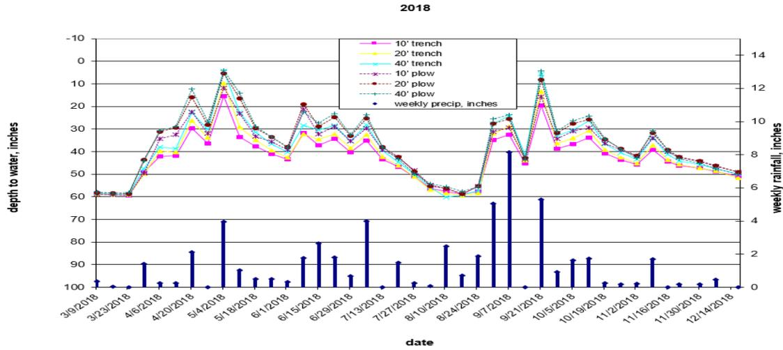
Figure 2. Water table and weekly precipitation in 2018 from two drainage installation methods at three distances.
