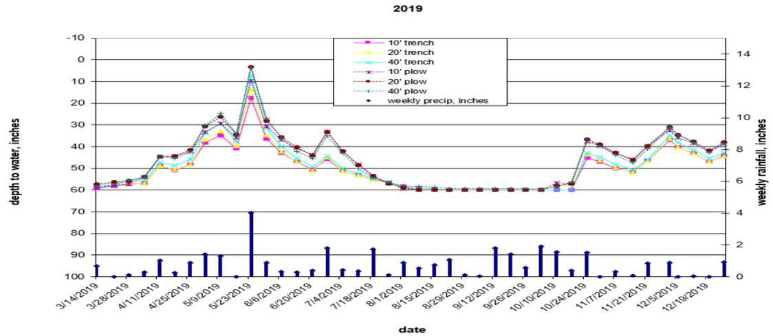
Figure 3. Water table and weekly precipitation in 2019 from two drainage installation methods at three distances.
