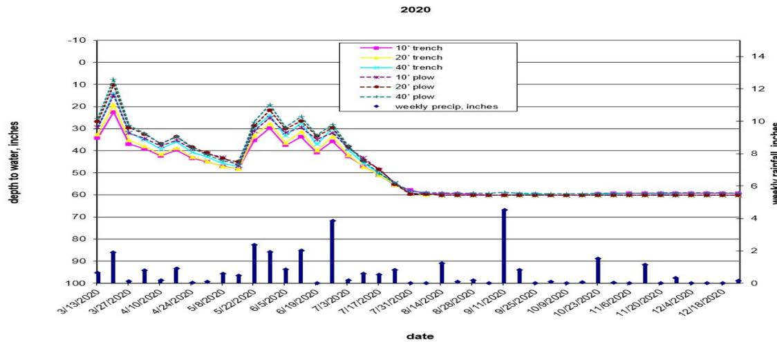
Figure 4. Water table and weekly precipitation in 2020 from two drainage installation methods at three distances.
