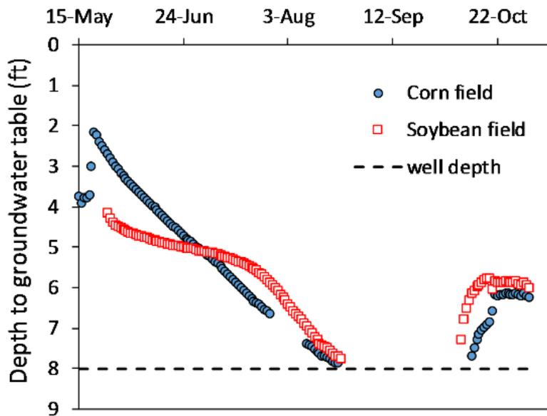
Figure 2. Water table depth with a well depth of 8 ft as indicated by the horizontal dashed line.
