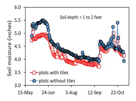
Figure 2. Soil moisture in plots with tile drainage (squares) and plots without tile drainage (circles) in 2017 at Crawfordsville, IA.
