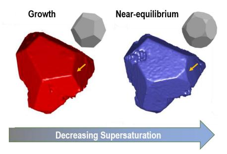
Figure 1. The growth and near-equilibrium shape of an icosahedral Al<sub>71</sub>Pd<sub>19</sub>Mn<sub>10</sub> quasicrystal.
