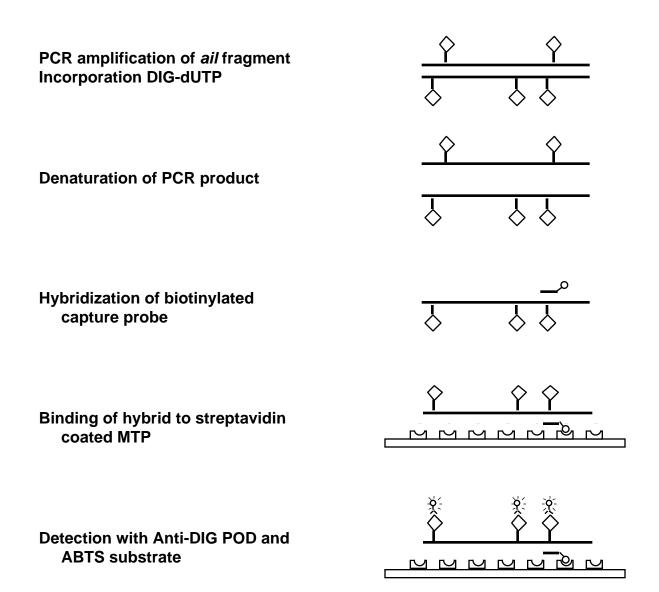
Figure 4 Schematic outline of the PCR ELISA procedure used to detect *Y. enterocolitica*. DIG-dUTP, Digoxigenin labeled dUTP; MTP, Microtiter plate; Anti-DIG POD, Peroxidase conjugated antibody against digoxigenin; ABTS, 2,2 '-Azino-di-[3-ethrybenzthiazoline sulfonate (6)].
