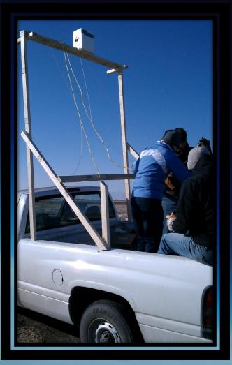
Reason for Test See if control of parachute is feasible Procedure Drop from aircraft and obtain flight profile Readjust control line to change angle of attack
