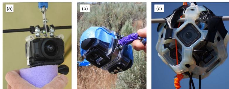
Figure 1. The cameras shown are ready for flight with hands and other objects included for scale. (a) Garmin VIRB 360 comes in its own housing. (b) Two Kodak PIXPRO SP360 cameras in the back-to-back dual camera housing accessory. (c) Six GoPro Session cameras in a WetHot360 mount.
