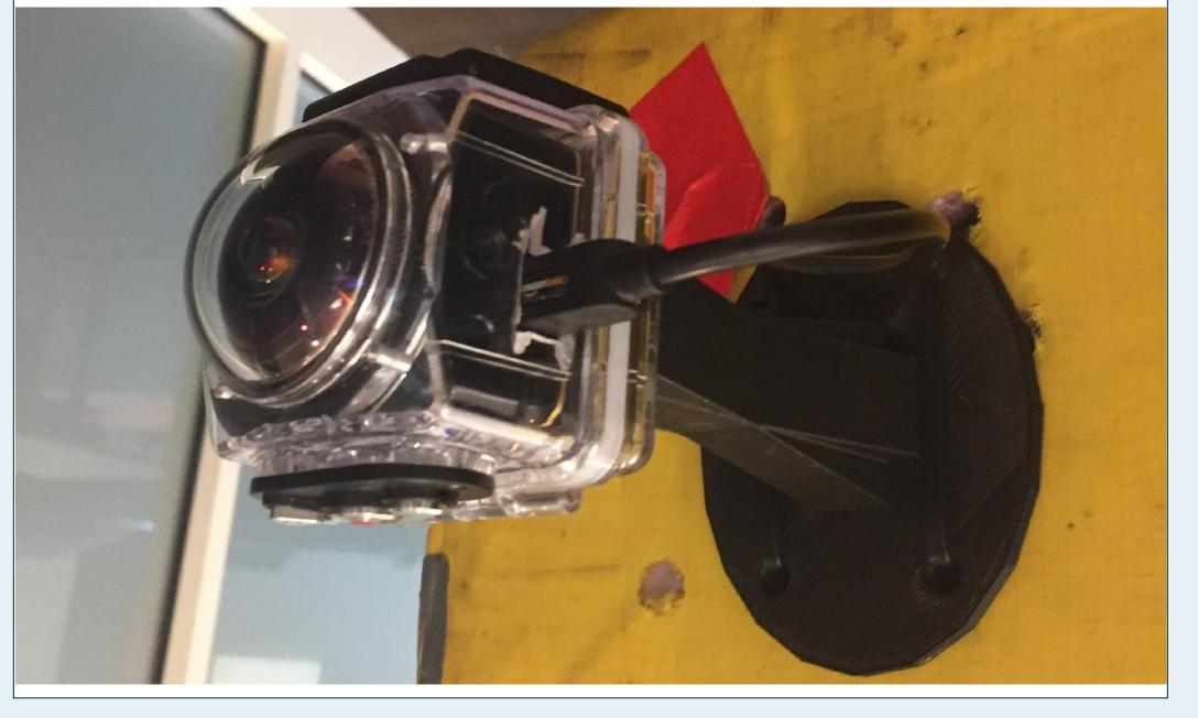
June 3, 2017. This flight primarily focused on testing the custom mount, which held up to a full flight and retrieval.
