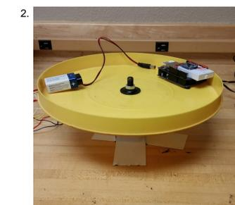
**Figure 2.** The table is coupled to a unipolar stepper motor. The motor is powered through a 12 volt power supply. The stepper motor is controlled by an Arduino Uno. There are two rotation calibration programs: 1) the table goes to a certain angular position and remains at that local, 2) the table rotates continually at a set rate.
