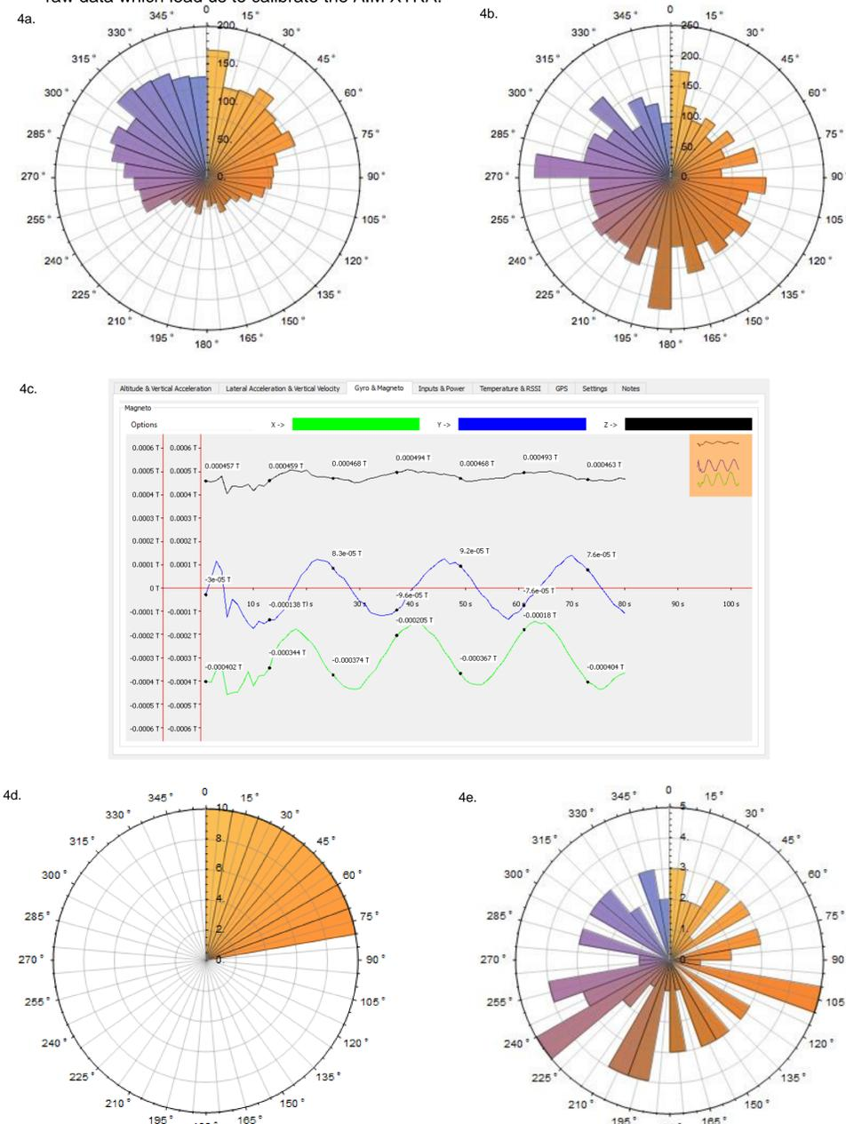
**Figure 4a.** Circular histogram of Arduino magnetometer continuously collecting run at .5 rev/s. Minimum bin count 29, max 168
