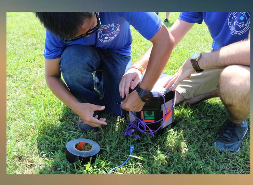
Preparing the line can be the most time consuming process during the ballooning process. Since line mass must be accounted for in the predictions, we cut our lines to length the day before a flight. Lines are secured to payloads by figure of eight knots for maximum strength and security. We also make sure that there is at least 15 ft. between parachute and the balloon to prevent parachute fouling.
