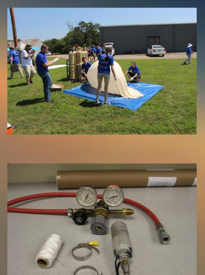
Our go-to setup for fill is: our inhouse machined fill nozzle, two pipe clamps, a two stage regulator, twine, a fish scale and some Gorilla Tape. Filling a 1600 gram balloon can be accomplished with about 10 people under normal conditions or two people and a tarp on a calm day. We had remarkably low surface winds that day so we went with the latter.
