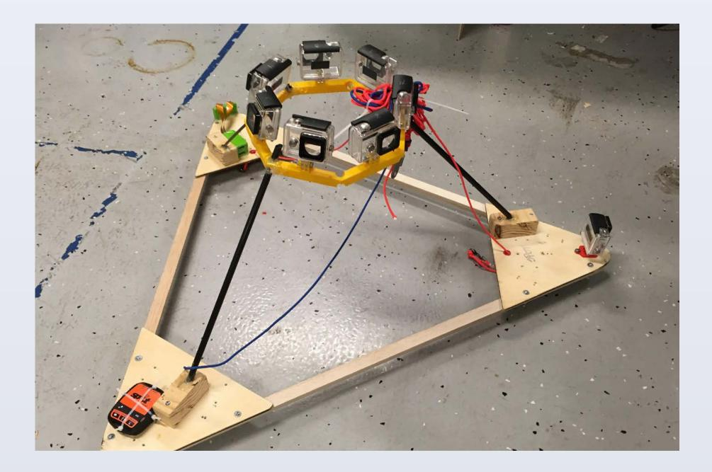
Based on previous designs from the University of Minnesota, stabilization paddles were made out of lightweight foam board and adhesive aluminum tape. By using aluminum tape, paddles acted as radar reflectors. Stabilizers were attached to solid carbon fiber rods, which extended ~30° horizontally downward from the bottom of the triangular base and glued to a wooden support using quick dry glue.
