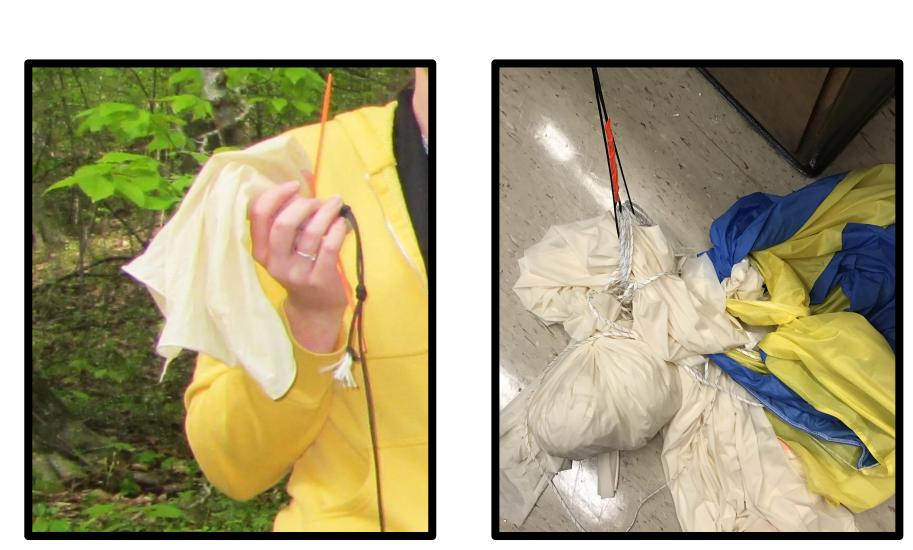
After balloon burst, a large amount of latex residue at the end of the leader line can interfere with descent and endanger payload survivability. The added weight and potential for entanglement from an incompletely disintegrated balloon can negatively impact parachute deployment and system recovery in a variety of ways. Our launch experience has taught us that the most robust balloon may not always be the best choice for a flight.
