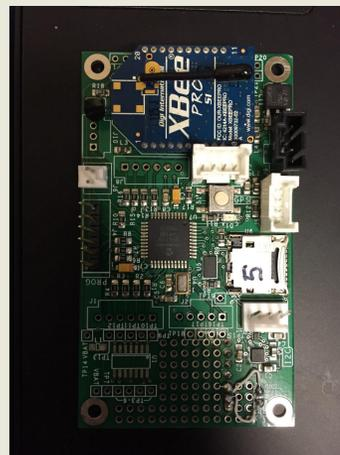
Figure 1: Trevecca's Pic Pod data logging board
