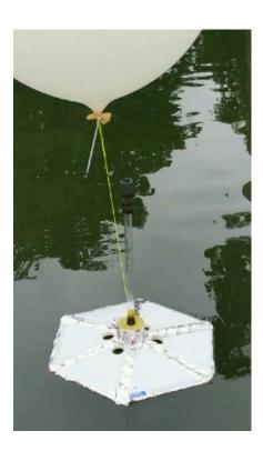
Fig. 11 The left picture shows the HydroChute with balloon as a sail. It successfully made it across the lake on its first maiden voyage. The right close-up picture hows the HydroChute floating above water with the payload and Globalstar link. The Clear shaft above can house the 900 MHz unit or a APRS Ham radio link. The four holes in the HydroChute are for parachute aerodynamic stability and for improving external temperature measurements with the higher flow.
