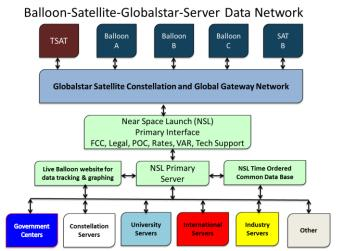
Fig 14 Block diagram of how data flows from various Balloon and Satellite systems through the NSL primary server and then to servers or log-on file data transfers to other institutions
