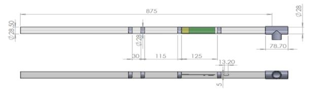
Fig. 5. CAD orographic views of LycPod-Mini unit showing some dimensions in mm.
