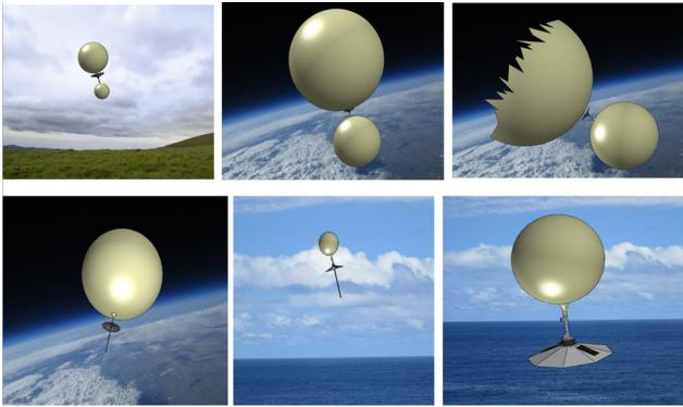
Fig. 9 CAD simulation showing launch, High altitude, Burst, Secondary balloon decent, Water approach, and hydro landing
