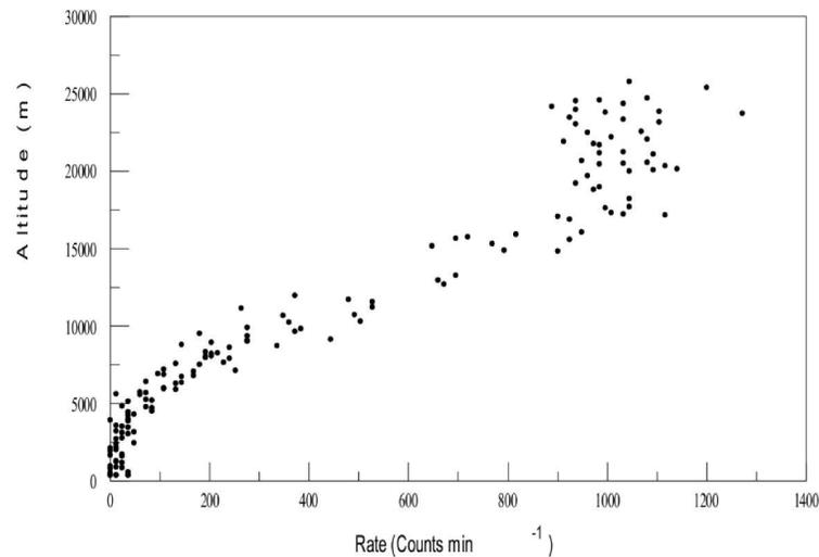
Figure 1. Altitude versus the omnidirectional count rate from an RM-60 GM tube for a balloon flight originating from Morris, MN, on 14 November 2009.
