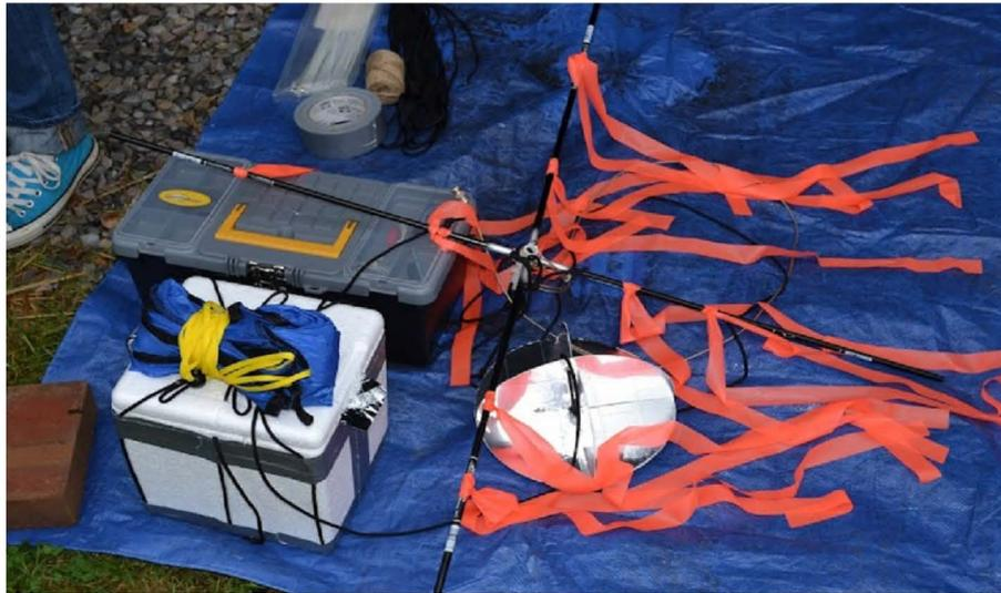
Figure 6: The launched payload and rigging. The payload is in the white box in the lower left with the parachute on top. The silver object in the center is the radar target and the orange streamers are tied to the crossed dipole transmitter antenna. It was hoped that the streamers would improve visibility if necessary to search for the payload but they did not survive the flight.
