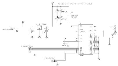
Figure 1. Schematic diagram of the Elktronics Iridium SBD9602 board.
