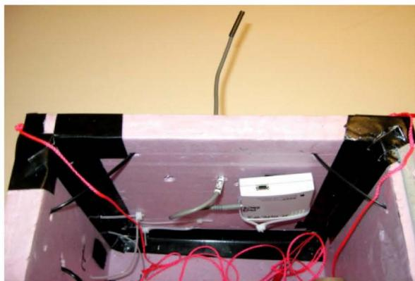
Figure 1: Typical installation of a U12 HOBO data logger and an Air/Water/Soil temperature sensor poking through the payload wall to measure the free-air temperature.
