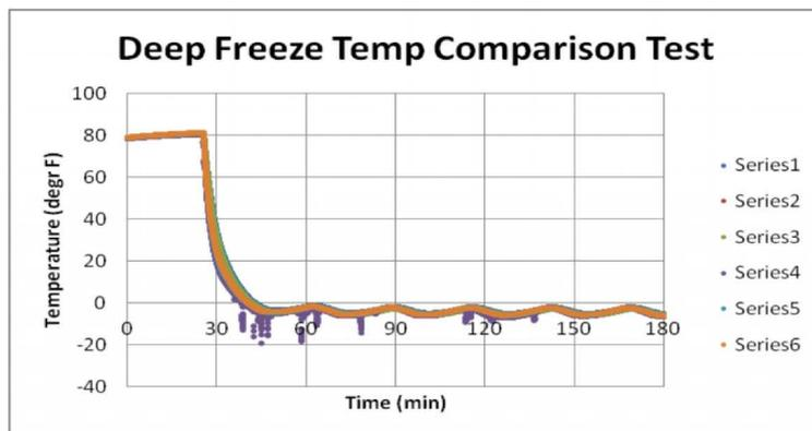
Figure 3a: Temperature response of 6 HOBO temperature sensors when placed in a deep freeze.
