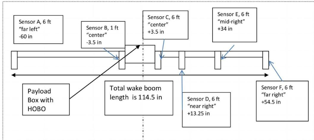
Figure 8a: "Wake Boom" schematic and dimensions.
