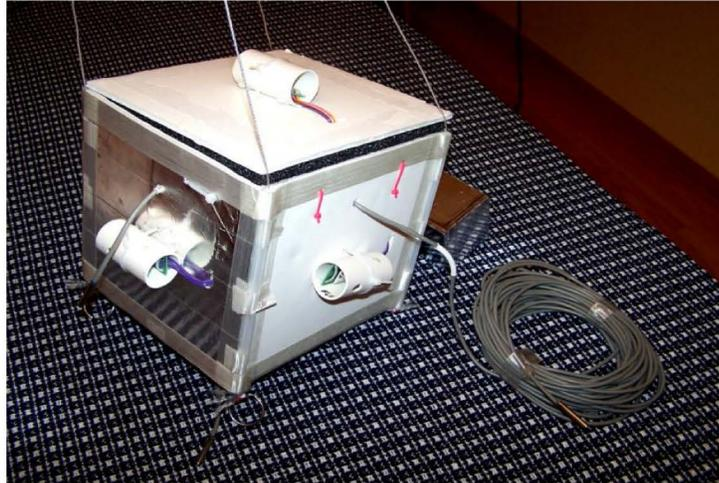
Figure 5: “Multi-colored” payload showing white side and silver side. The other sides were black and pink. HOBO thermometers, some shaded (not shown) and others exposed, some dangling many feet below the payload were used to study how the presence of the payload itself affected the recorded temps.
