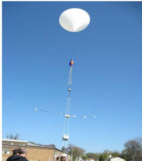
Figure 8c: The wake boom ready to be launched.
