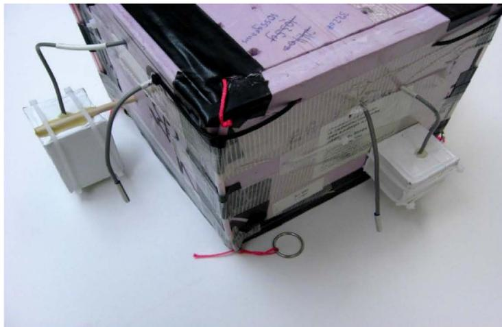
Figure 6: St. Catherine University payload with exposed temperature sensors (2) plus sun shielded sensors, one on a boom.
