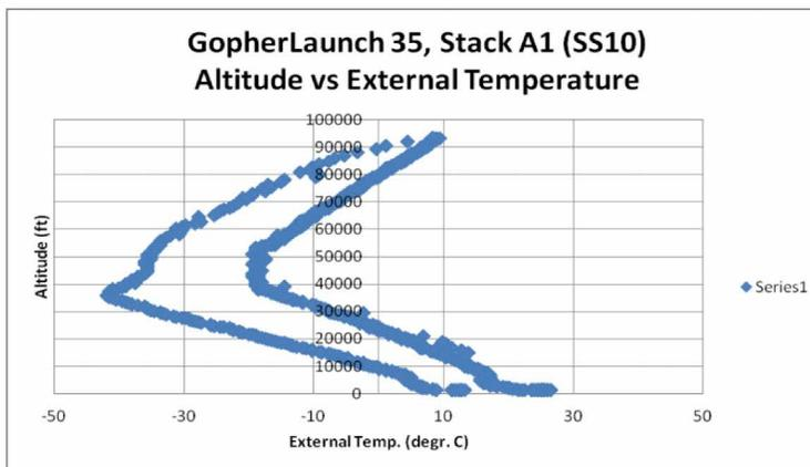
Figure 2b: The same external temperature data but plotted versus altitude instead. Ascent data is on the right; descent data is on the left.
