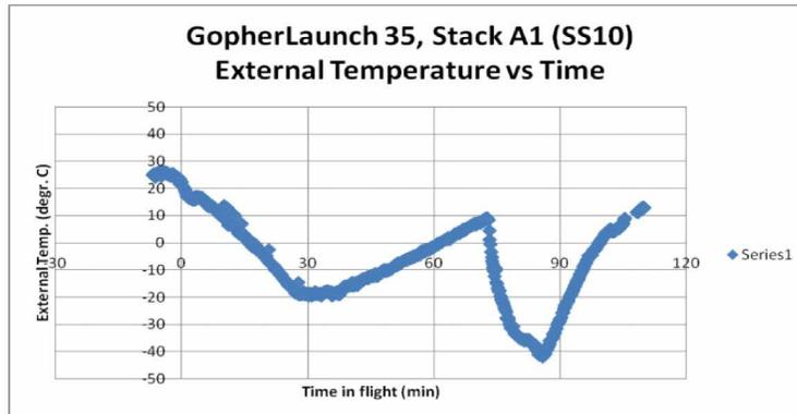
Figure 2a: External temperature versus time during a U of MN high-altitude balloon flight.
