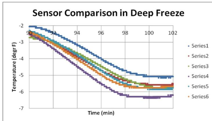
Figure 3c: Zoom-in comparison of sensor readings at freezer temperature, showing a different order.
