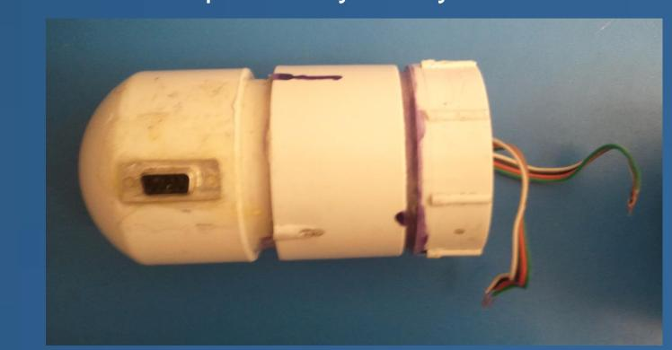
The second version, which was built and is pictured above, is essentially a scaled-down version of the first concept. The Arduino and camera were moved out of the chamber, and the crickets would be viewed through a Plexiglas window. The internal heater and sensors would be connected with electrical feed-throughs in the chamber wall.
