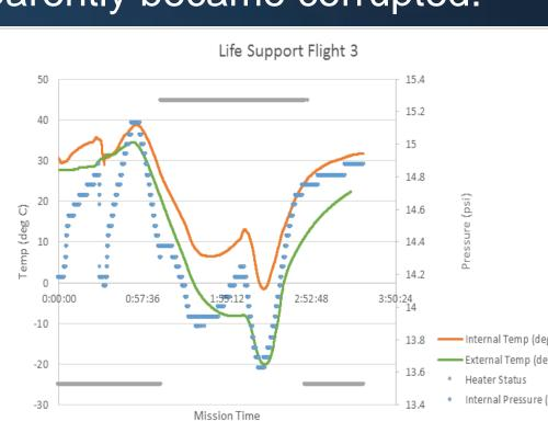
The second flight was much more successful, with the crickets (and sowbugs included on this flight) surviving. However, the camera overheated just before launch, so no video was recorded. On the third flight, flown without insulation, the heater was not quite capable of keeping up with the low external temp. so the internal temp. dropped to just below freezing. Despite this, the crickets still survived.
