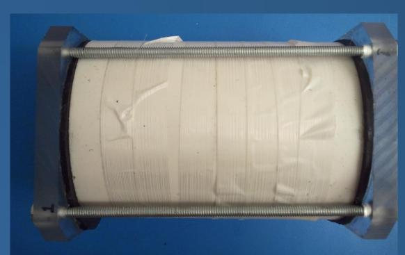
Our final flight canister (shown above) was based on a design for a "High Altitude Test Chamber" by H. Brooks at DePauw University (www.tinyurl.com/basedepauw). It consisted of a (tape-wrapped) section of 4" diameter PVC pipe, with Plexiglas plates at either end. Threaded rods with nuts were used to tightly compress the Plexiglas plates on rubber gaskets to the ends of the pipe. Silicone-based vacuum grease was applied to the gaskets.
