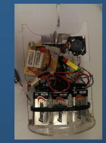
For the first flight, the electronics, batteries, and cricket holder were simply hot-glued in place. However, turbulence just after burst led to the glue attachments failing. In later flights a removable 'sled' for mounting electronics was built from laser-cut acrylic sheets (see above).
