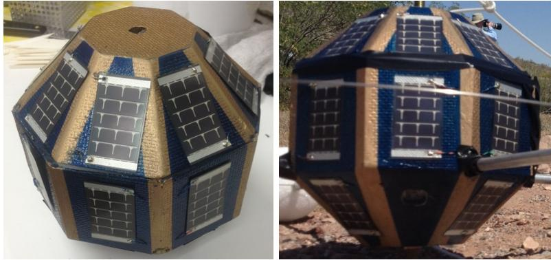
Figure 2. Sun sensor implementation on payload.
