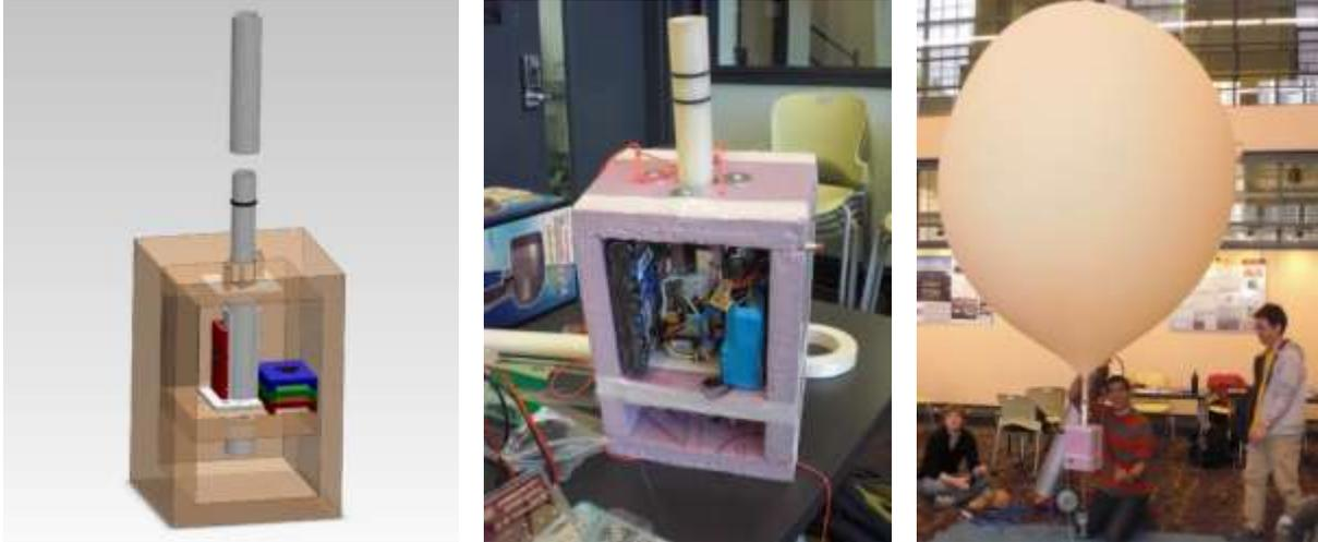
**Figure 2.** (a) CAD of vent mechanism within a payload shell, controlled by an Arduino (in blue, lower right). (b) The actual vent payload, with a downlink ZigBee radio module (blue, lower right), and a serious battery pack (on the left) to power the nichrome burner cut-downs. (c) Ground testing of the Float payload attached to the neck of a tethered balloon indoors.
