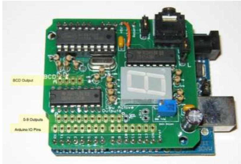
**Figure 1. A DTMF decoder-only shield. DTMF tones fed in through the audio jack (upper right) are displayed on the 7-segment display and available to the Arduino microcontroller (below the shield). Our implementation also used a SD-card shield to log incoming DTMF commands plus an XBee radio shield to relay commands on the XBee network. Photo from Ref. 1.**
