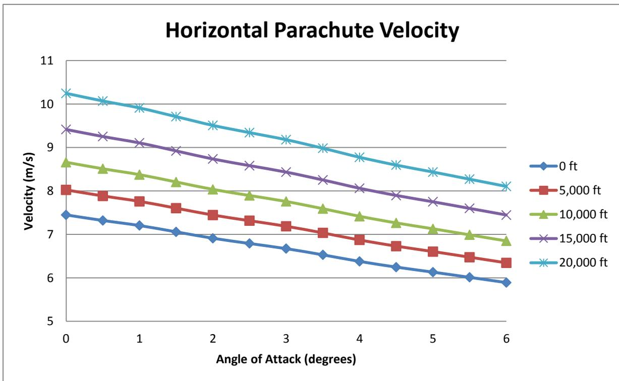
Figure 19: Estimated Parachute Horizontal Velocity At Various Altitudes And Angle Of Attacks
