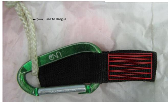
Figure 25: Drogue attachment point on ram air parachute
