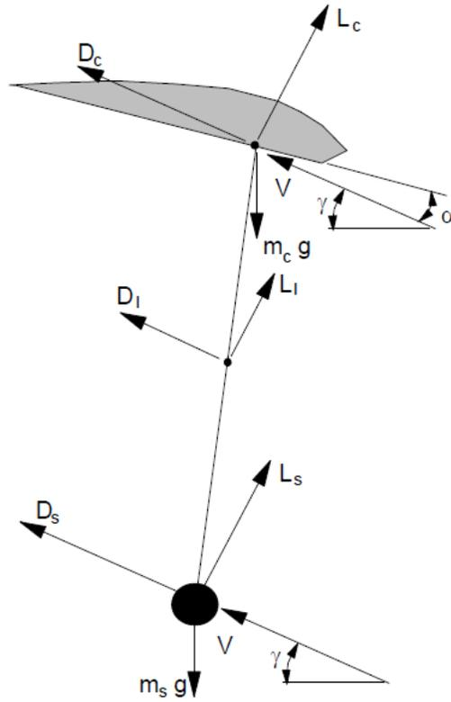
Figure 17: Ram Air Parachute in Steady, No Wind Glide
