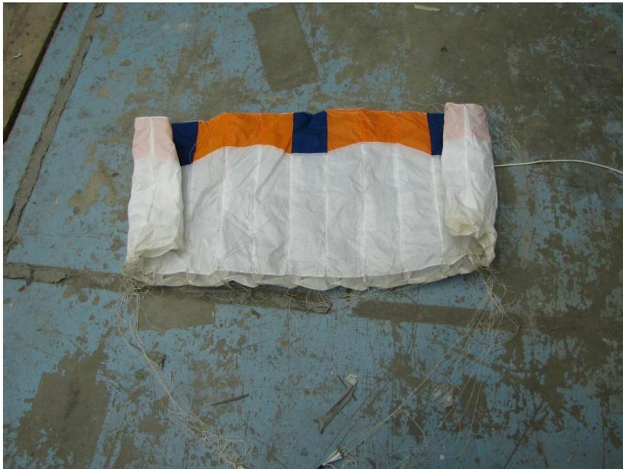
**Figure 22: Parachute is folded inwards in sets of 2 cells**
