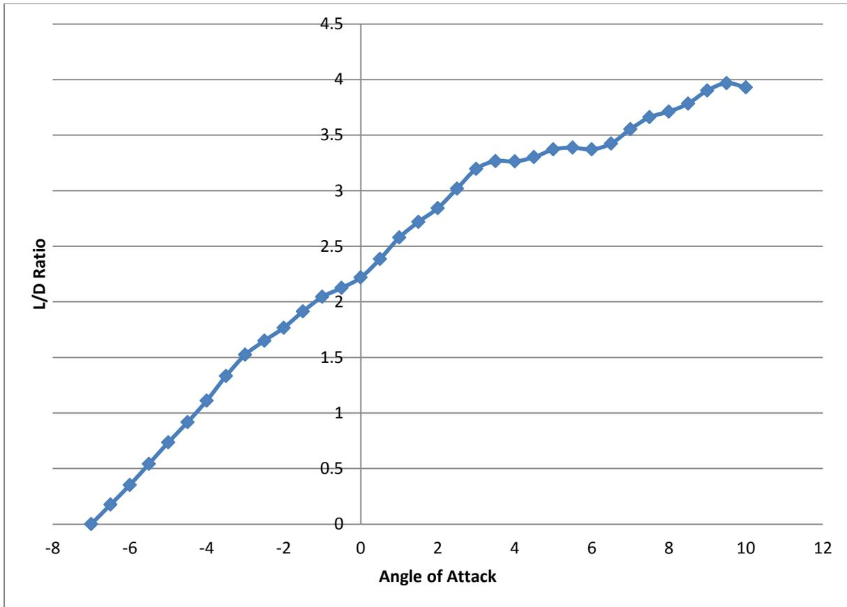
**Figure 16: Theoretical Lift to Drag Ratio for Selected Ram Air Parachute**
