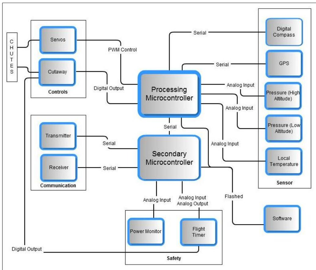
**Figure 2. Electrical System Block Diagram.**
