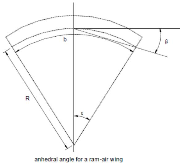
Figure 14: Anhedral Angle for Ram Air Parachute
