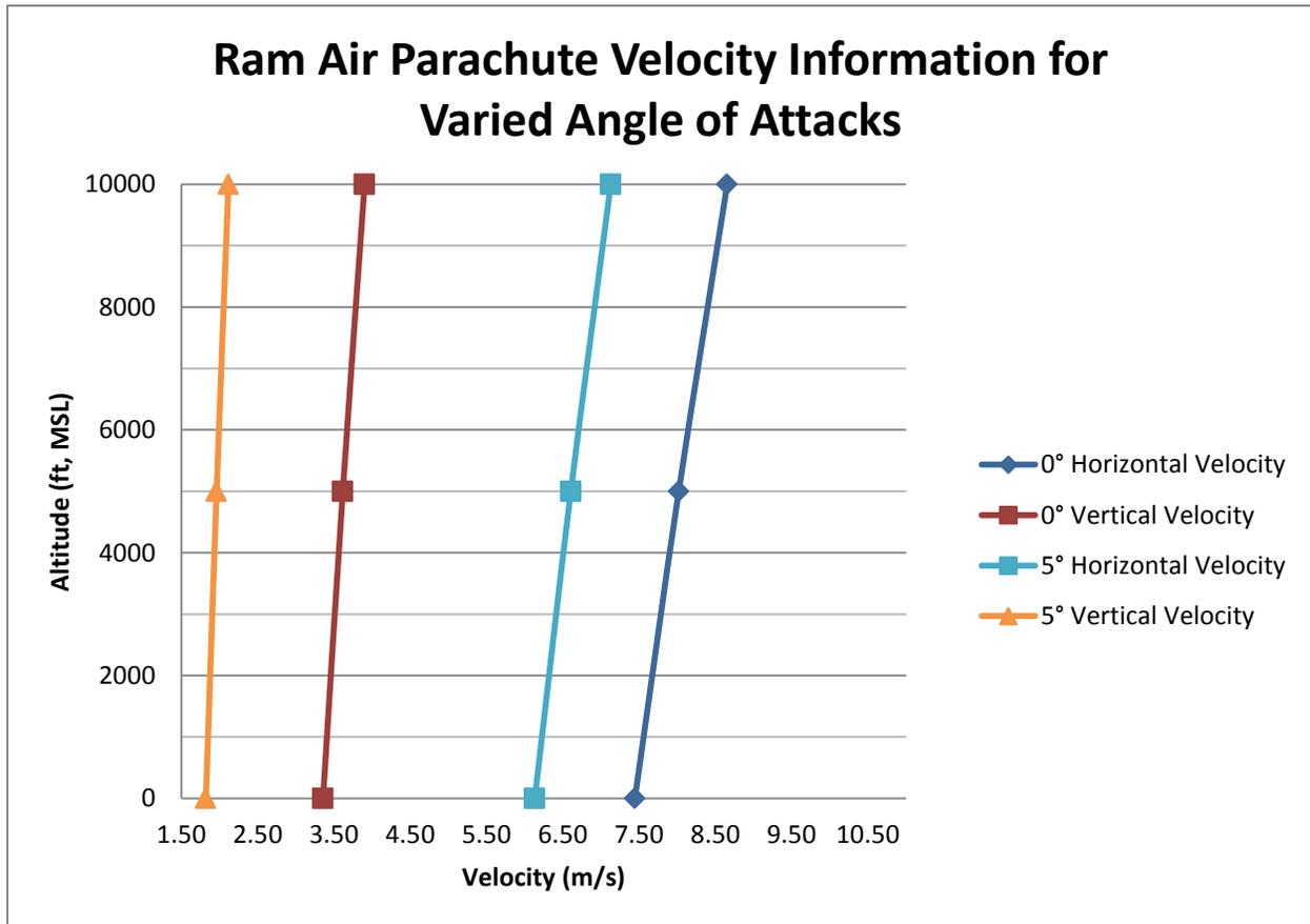
Figure 24: Estimated parachute velocities at 0° and 5° angle of attacks from 10,000 ft to sea level
