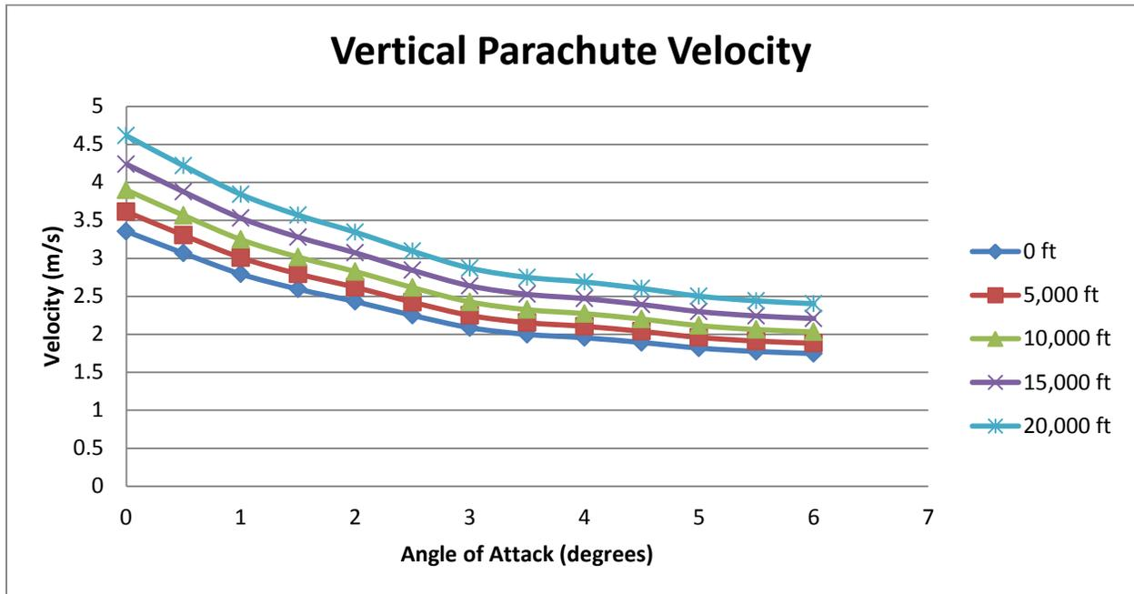
Figure 20: Estimated parachute vertical velocity at various altitudes and angle of Attacks
