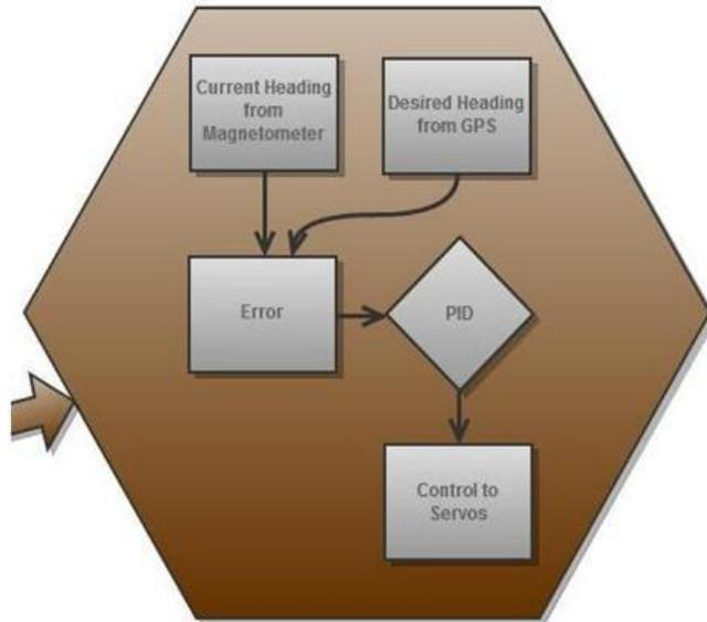
**Figure 10. Main Parachute Steering Routine**
