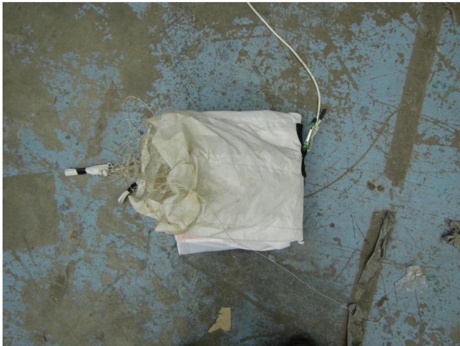
**Figure 24: Parachute folded to its final folded setup**
