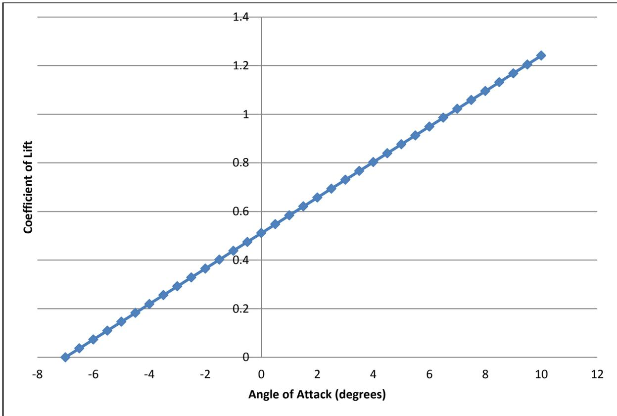
Figure 13: Theoretical Coefficient of Lift for Selected Ram Air Parachute
