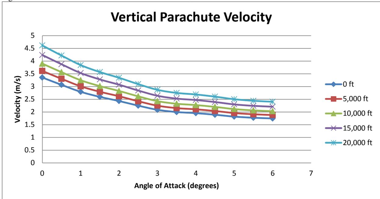
Figure 20 displays the estimated vertical velocity the parachute at a given velocity and angle of attack.
