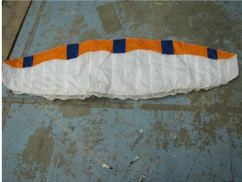
**Figure 21: Parachute is laid flat with lines strung out**
