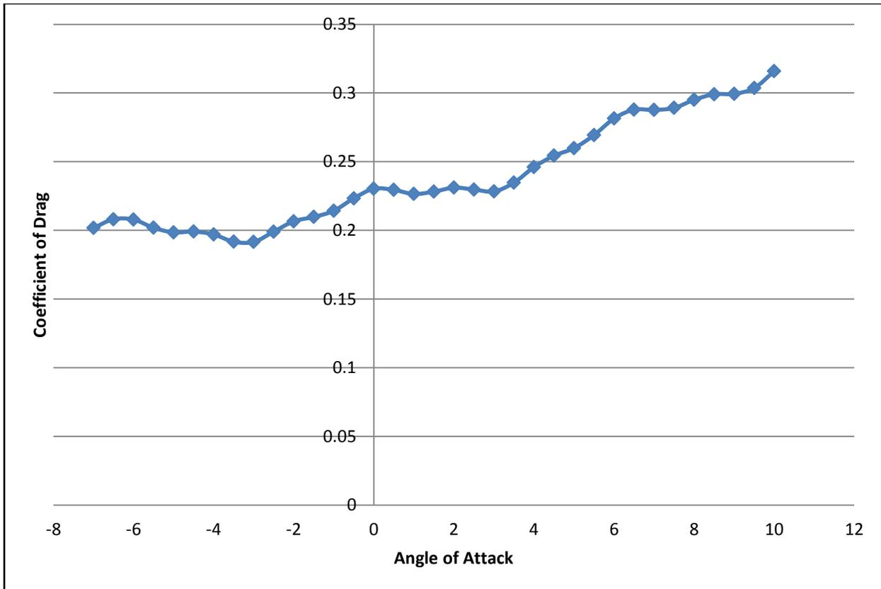
**Figure 15: Theoretical Coefficient of Drag for Selected Ram Air Parachute**
