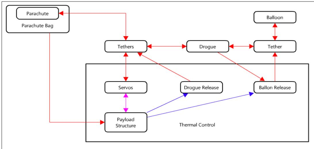
Figure 1. Mechanical Systems Block Diagram
