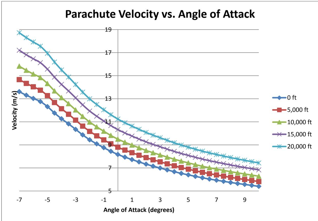
Figure 18: Parachute Velocity At A Given Angle Of Attack And Altitude
