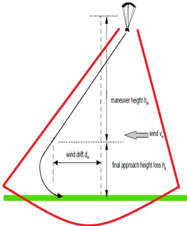
Figure 11: Precision Aerial Delivery System Principle
