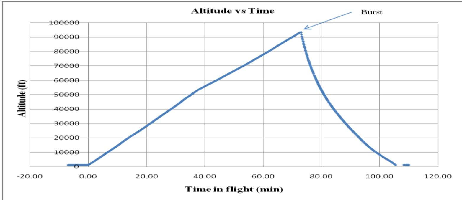
The Altitude (in feet) versus Time (in minutes) graph of the balloon flight for stack A2.
