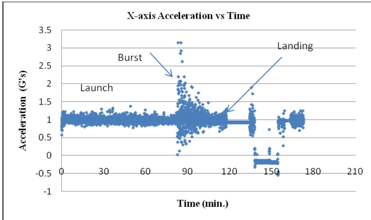
The x-axis acceleration (in G's) versus time (in minutes) graph during all stages of flight from the Columbia Height's payload.
