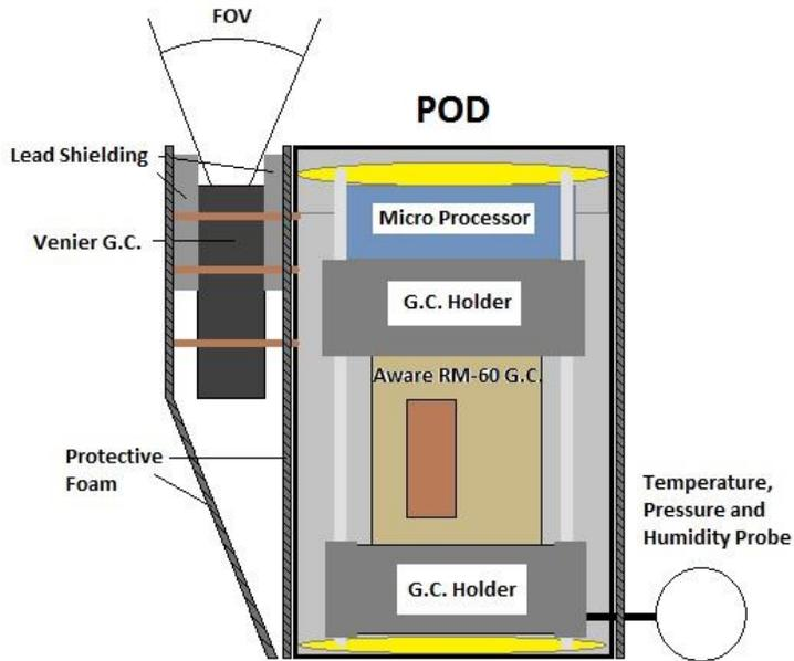
**Figure 3. POD Contents.** The arrangement and contents of the POD that was flown on the night launch.
