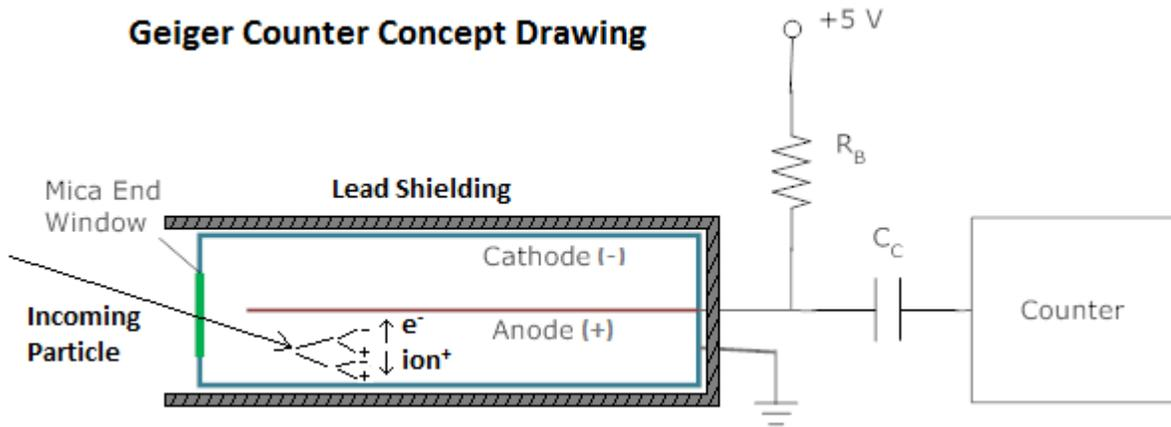
**Figure 7. Concept Drawing.** Particles enter through the Mica End Window and create electron-ion pairs by collisions with gas molecules. Electrons are attracted to the positive anode, creating a current.
