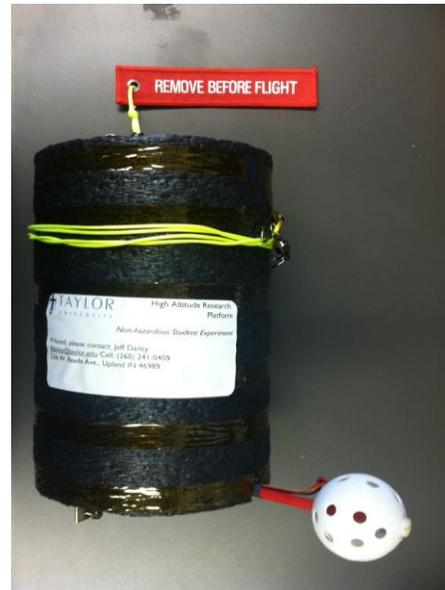
**Figure 4. Final Product.** The POD wrapped in foam before launch.
