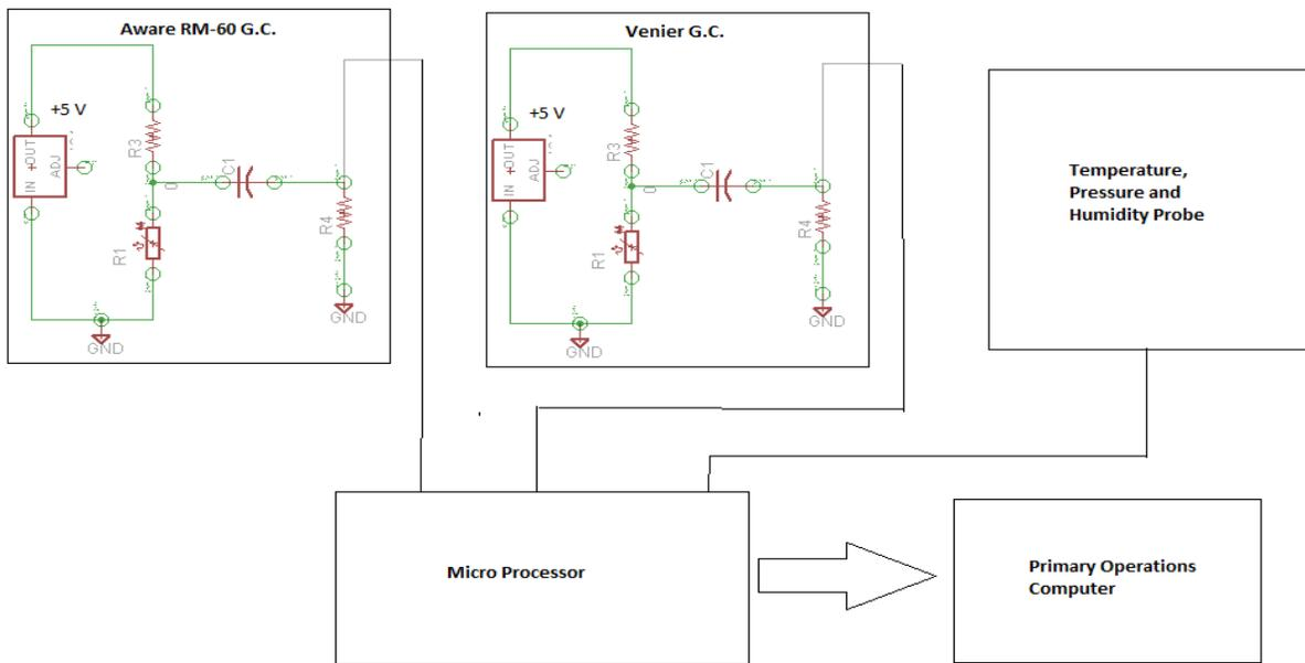
**Figure 6. System Interface Layout.** Block diagram of the Geiger counters and sensor probe interfacing with the microprocessor.
