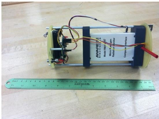
**Figure 5. POD Interior.** The inside of the pod with RM-60 Geiger counter held by base.
