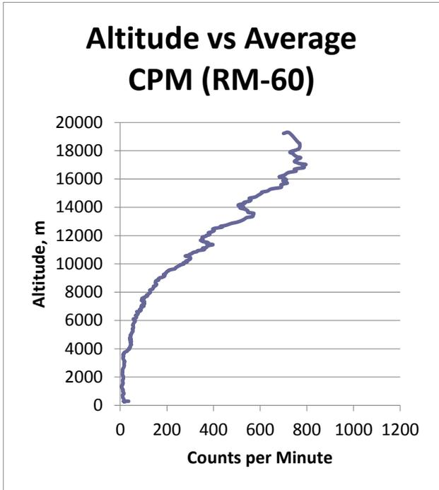
**Figure 8. Altitude Plot.** (Left) The data from the daytime launch using the RM-60 G.C on March 9, 2013.
