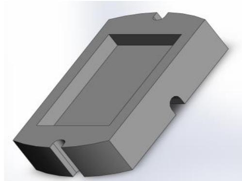
**Figure 2. Geiger counter Base.** Design of Geiger counter base generated in SolidWorks and printed on 3D printer.
