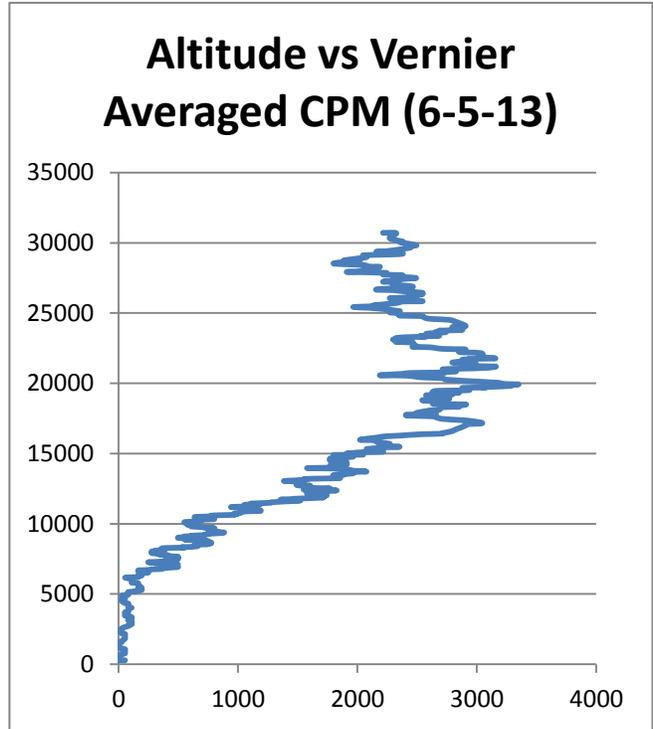
**Figure 11. Altitude Plot.** The final daytime launch data collected by the Vernier GC on June 5, 2013.
