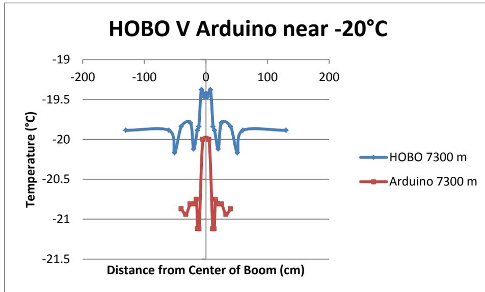
**Figure 10A:** Comparison plot of two temperature sensor systems at 7300 meters, reading a temperature of -20 Celsius, during an ascent.
