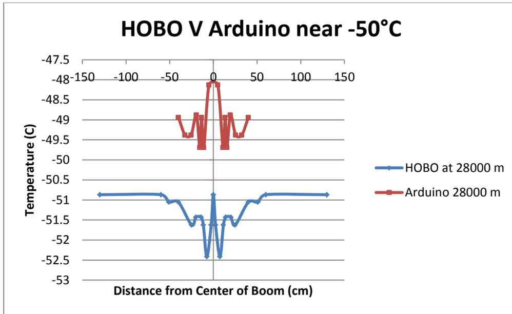
**Figure 10C: Comparison plot of two temperature sensor systems at 28,000 meters, reading a temperature of -50 Celsius, during an ascent. This graph is near burst.**
