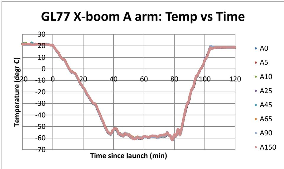
Figure 15A. Temperature of the 8 sensors on the A arm during flight 2X. The temperature in the stratosphere was fairly constant above the tropopause and the temperatures at different parts of the boom did not vary from one another nearly as much as during flight 1X.
