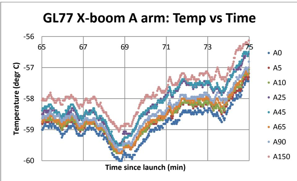
Figure 15B. A zoom-in of the data late in the ascent for flight 2X. There is a persistent difference in readings between temperature readings, but it was not in the expected (spatial) order.
