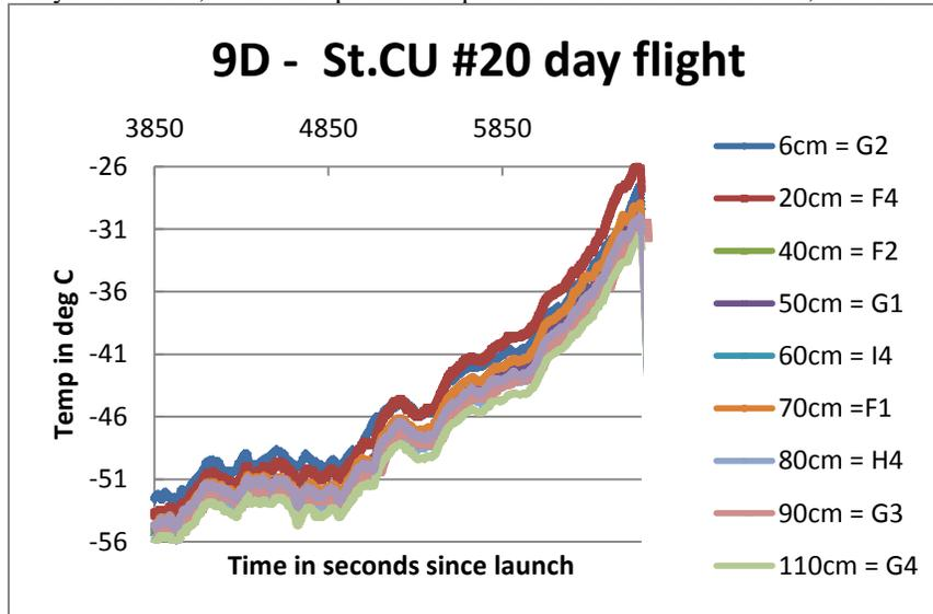
**Figure 5. Graph showing HOBO temperature sensors values vs. time for a daytime flight conducted on 10-26-2013 – the data encompasses a latter portion of ascent plus a small portion of descent data.**
