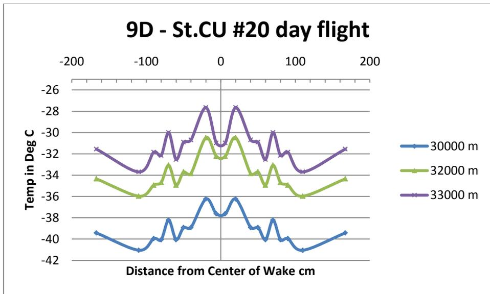
**Figure 6. Temperature vs. distance from center of boom and how wake profile varies with altitude during a day flight.**
