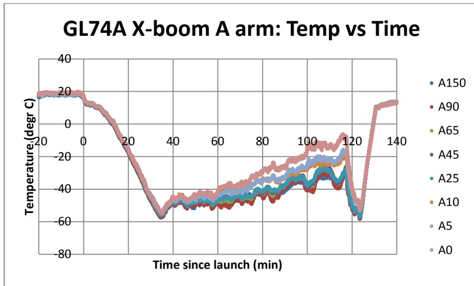
**Figure 11. Temperatures from 8 sensors on one arm of the X-boom during Flight 1X. The temperature differences in the stratosphere were much larger than expected and may be due in part to the proximity of the payload box enclosing the Arduino data loggers.**
