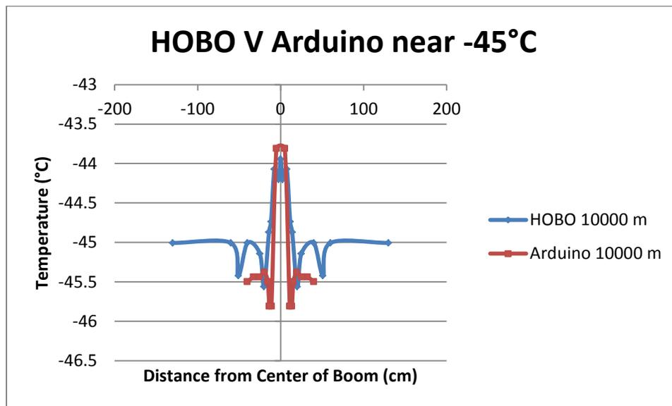
**Figure 10B:** Comparison plot of two temperature sensor systems at 10, 000 meters, reading a temperature of -45 Celsius, during an ascent.
