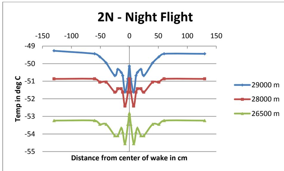
**Figure 9.** Distance from center of boom and how the HOBO recorded temperature is different at those positions at 3 different altitudes.
