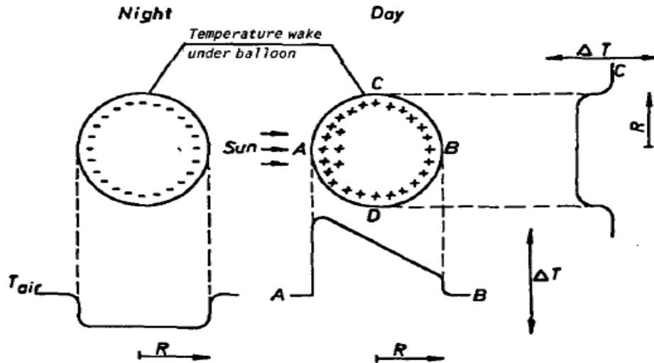
Figure 2. Symmetrical (Asymmetrical) temperature of balloons and thermal wakes during Night (Day) ascents. Figure reproduced from Ref. 5.
