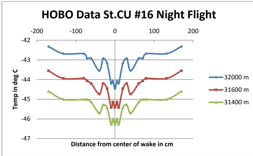
**Figure 8.** Distance from center of boom and how the HOBO recorded temperature is different at those positions at 3 different altitudes.
