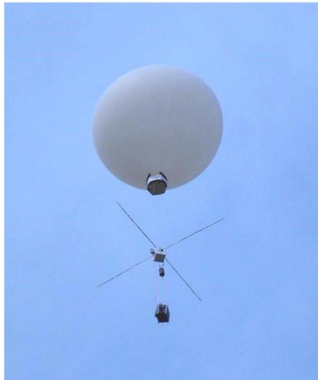
**Figure 4.** The X-boom on flight 1X, tied to the parachute basket attached to the neck of a 3000-gram Kaymont weather balloon.
