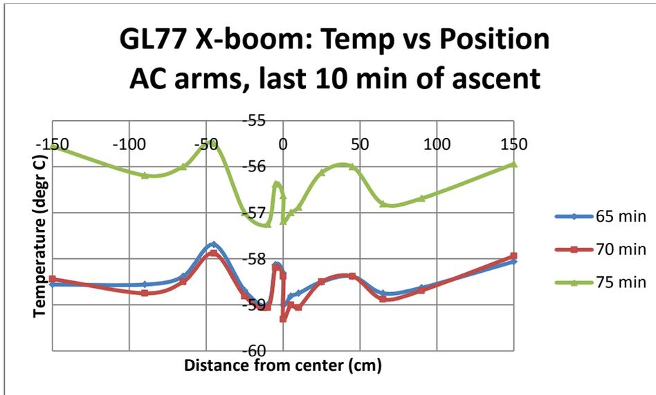
**Figure 16.** Attempting to image the thermal wake using sensors on arms A and C late during the ascent during Flight 2X. The structure here has a surprising shape but seems to persist over the full 10 minutes. This may be due to calibration differences between the sensors rather than to the wake effect.
