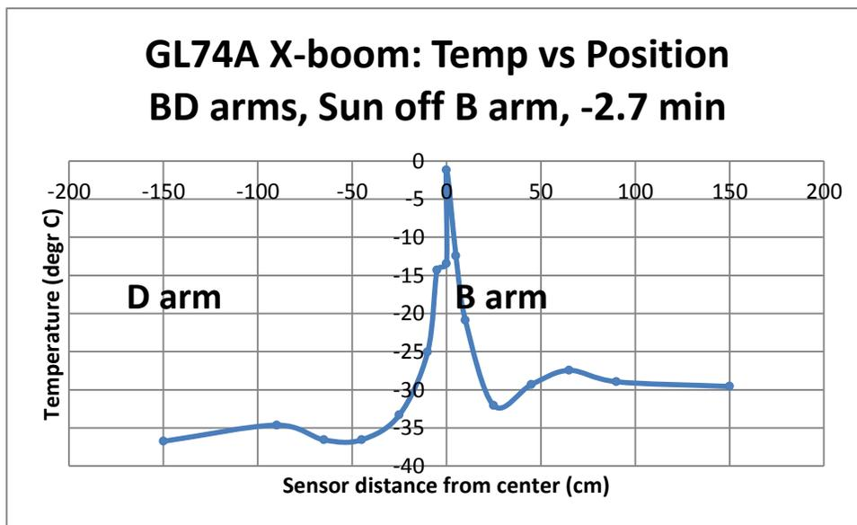
**Figure 12.** Temperature profile along the BD-arm line of the X-boom (A) when the sun was off arm A, less than 1 minute before burst and (B) when the sun was off arm B, about two minutes earlier. The central temperature spike may be more than just a wake effect. Wake asymmetry is expected at time (B) but not at time (A), but both appear similar. The unexpected temperature asymmetry on the outer ends of arms might be due to the shadow of the balloon falling on the arms of the boom.
