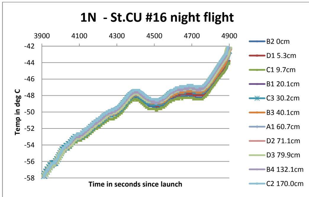
**Figure 7. Graph showing HOBO temperature sensor values vs. time for a nighttime flight conducted on 8-1-2013 – the data encompasses a latter portion of ascent plus burst.**
