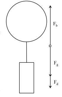
Figure 1. The force balance of the balloon on ascent.
