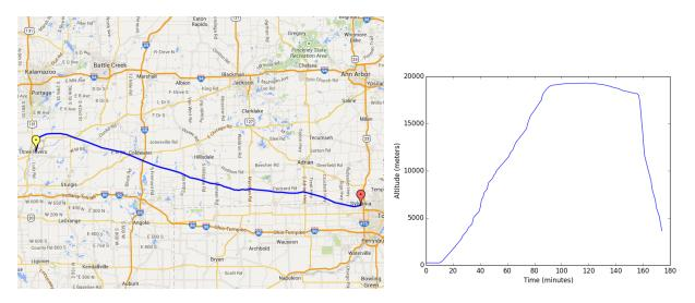
Figure 7. The left plot show the actual flight path of the zero pressure balloon launched on April 12, 2014. The right figure shows the altitude as a function of time for the balloon.
