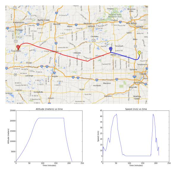
Figure 6. Predictions for a zero pressure balloon launch that was conducted on April 12, 2014. The top plot shows the horizontal path that was predicted, while the lower left plot shows the predicted altitude and the lower right plot shows the wind speed as a function of time that the balloon was predicted to encounter.
