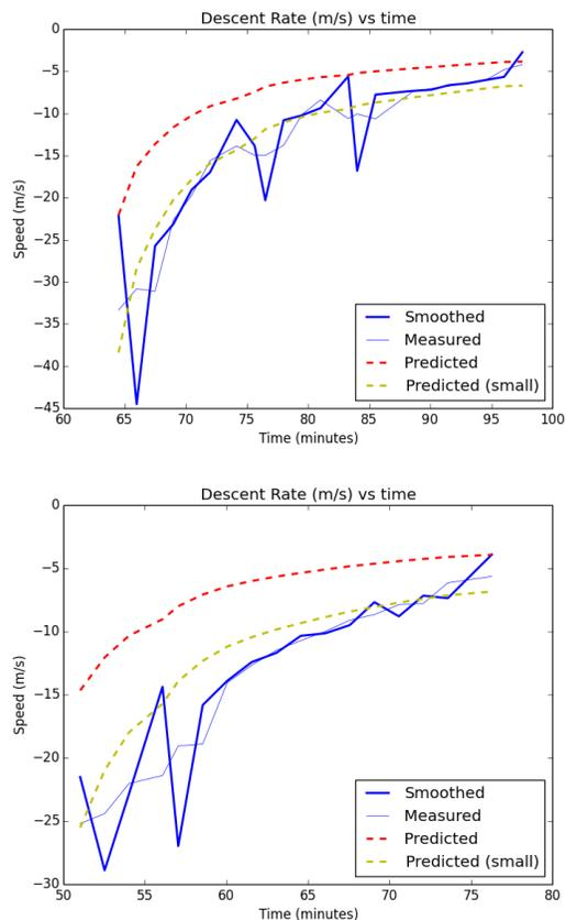
**Figure 4.** Descent rate predictions (red dashed line) and measurements (blue solid lines) for the two different flights.
