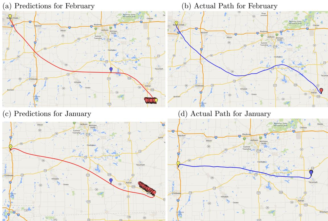
**Figure 5.** Predictions (left) and actual flight paths (right) for the February 2014 (top) and January 2014 (bottom) launches. The yellow pin shows the launch site, the blue pin shows the burst location, and the cluster of red (and one yellow) pins show possible landing locations. On the right, the yellow pin marks the launch site, while the pin other pin indicates the actual landing site. These are direct outputs from the web page.
