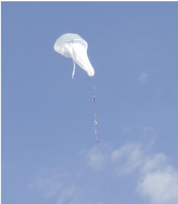
**Figure 8.** A zero pressure balloon a couple of minutes after launch.
