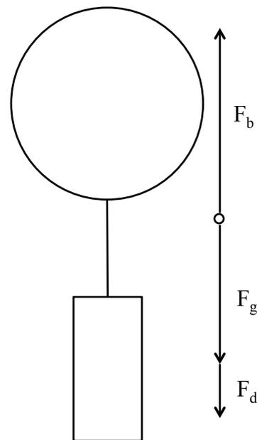
Figure 1. The force balance of the balloon on ascent.
