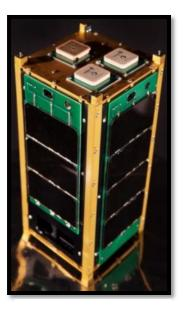
Fig. 4 TSAT dual Cubesat
