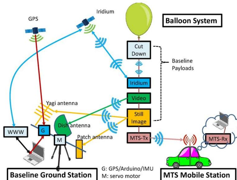
Figure 2. Functional diagram of the solar eclipse ballooning system
