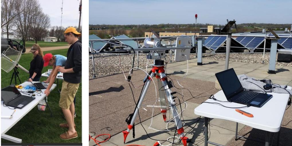
**Fig. 5.** On the left – “up-range” (i.e. at launch site) ground station to communicate with the FreeWave MMT-2 radio in SPARTA. On the right – “down-range” (i.e. near predicted burst location) ground station ready (but unable) to communicate with the RFD900 radio in CSI.
