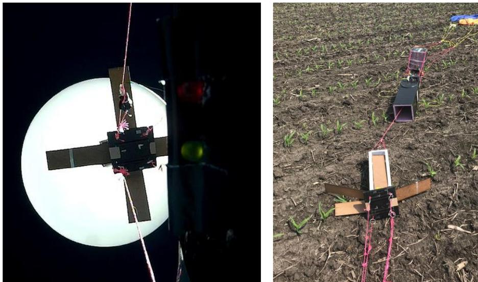
**Fig. 10.** On the left – Still photo from an up-looking video showing MOC-SOC post-deployment during flight. Camera was mounted on the side of a payload so the image is partially obscured. On the right – MOC-SOC after landing, with extended “solar” panels, below the mock P-POD.
