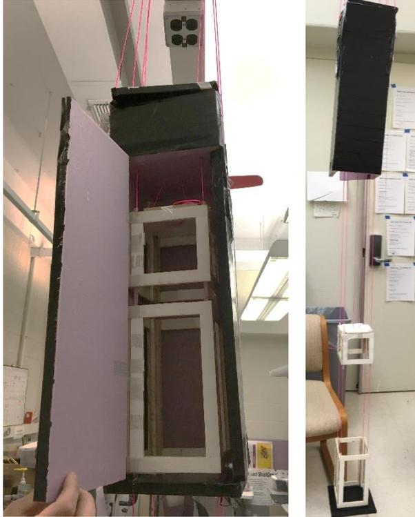
**Fig. 7.** On the left – mock CubeSat “cases” for padding (not thermal) protection plus tubing for standard balloon payload rigging. On the right – after deployment from the mock P-POD the cases (empty in this test), plus bottom cover, slide down rigging lines (toward payload below).
