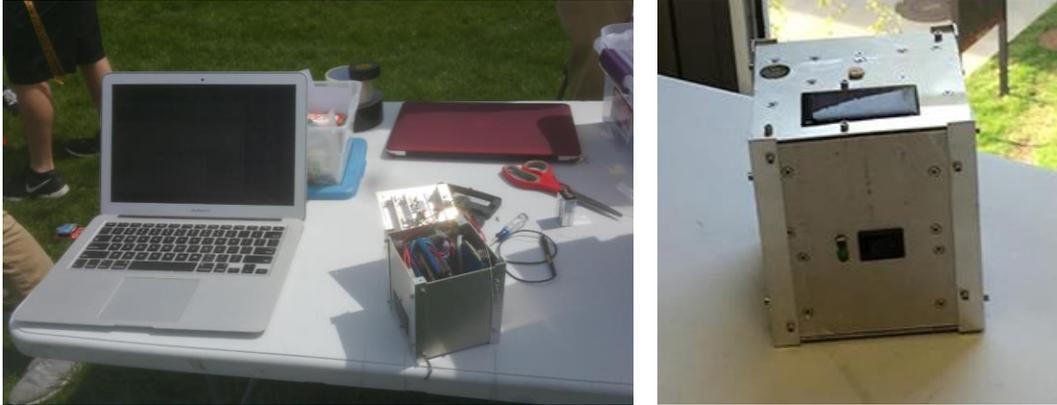
**Fig. 1.** “Modulus” – a 1U mock CubeSat with an all-aluminum shell containing a Razor M0 9-degree-of-freedom IMU/microcontroller, Geiger counter, multiple other sensors (see list in text), body-mounted solar panels, and an XBee (short range) radio for data telemetry to the ground through a nearby “Comms” radio-relay payload flying on the same balloon stack.
