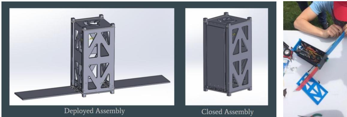
**Fig. 3.** “SPARTA (Solar Panel and Radio Testing Artifice)” – a 2U mock CubeSat that was entirely 3D printed containing an AIM XTRA commercial gps-enabled rocketry altimeter plus a FreeWave MMT-2 (long range) radio to communicate with a ground station at the launch site. SPARTA had two panels which deployed in flight, on which were mounted solar cells.
