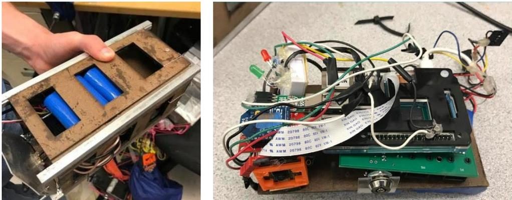
**Fig. 2.** “CSI (Camera Satellite Initiative)” – a 2U mock CubeSat with MDF walls and aluminum corners containing a Raspberry Pi miniature computer with Raspberry Pi camera, RFD900 (long range) radio, and an XBee (short range) radio. CSI is essentially a re-mounting in a 2U form factor of the “still image payload” developed by the MT Space Grant for the Space Grant Eclipse Ballooning Project modified by the MN Space Grant to serve as a communications relay [Ref.3].
