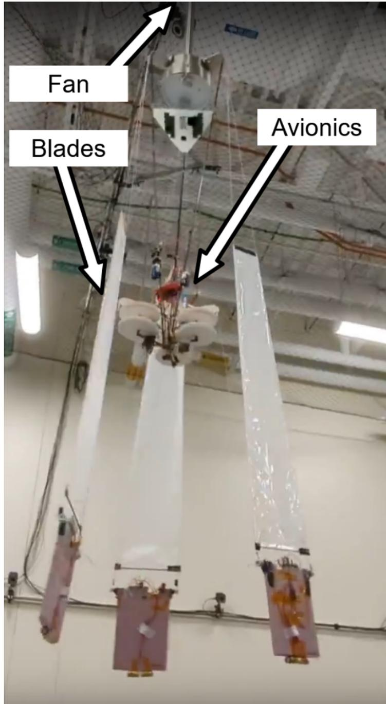
**Fig. 3.** Full V4 prototype hanging in the ASPEN Lab ready for testing. Note the blade tips, which were used for previous versions, are inactive and only used as tip weight. Overall, the device weighs approximately 1.7 kg in its current configuration.
