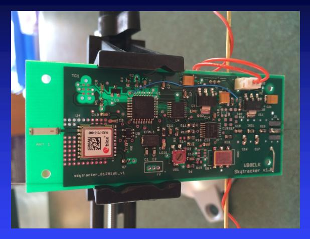
Designed a board called the Skytracker. Complete tracker with onboard GPS that can transmit on VHF or HF frequencies. APRS or WSPR modes.
