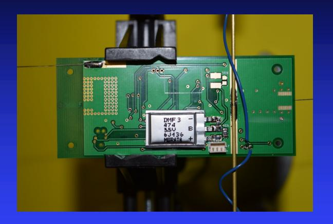
The 0.47 Farad Supercap on the back is very lightweight.
