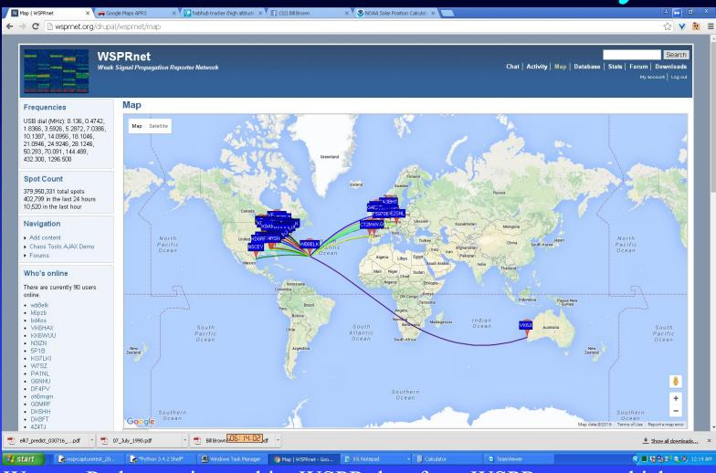
Wrote a Python script to skim WSPR data from WSPRnet.org which reformats it to post to the vehicle tracker websites. Data received as far as Australia from the tiny 20 milliwatt HF transmitter.
