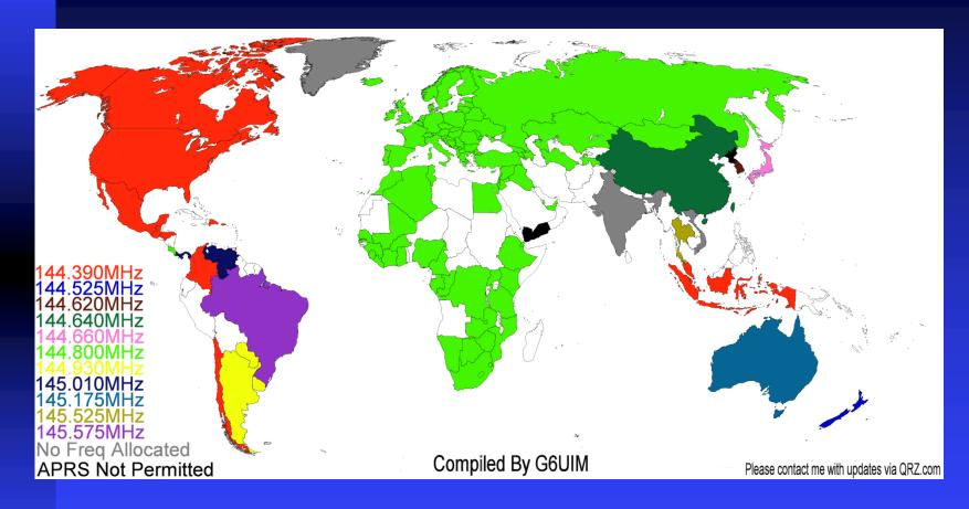
For an APRS tracker you have to automatically switch frequencies based on your location in the World.
