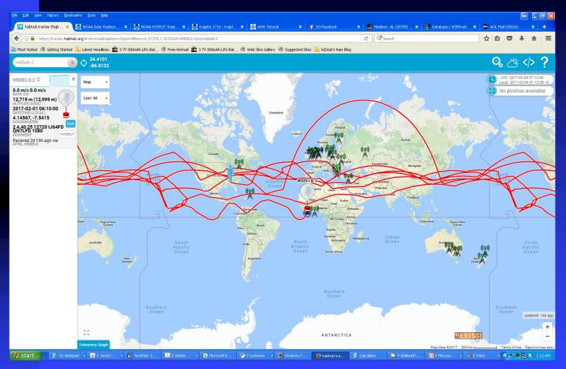
WB8ELK-6 WSPR Skytracker 20m WSPR flight went around the World over 6 times after flying at 40,000 feet for 75 days.
