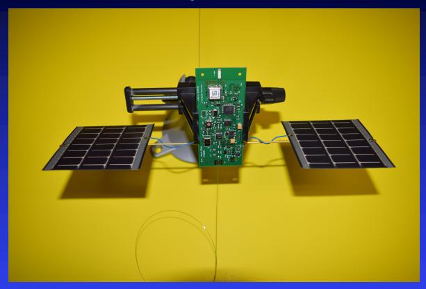
Totally solar-powered using very lightweight thin-film flexible solar cells by PowerFilmSolar. Guitar string antenna wires. Magnet wire for WSPR version.
